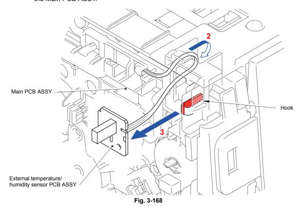
Harness routing: Refer to " 2 External Temperature/Humidity Sensor PCB ASSY,
