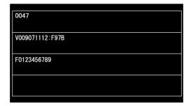
The main firmware version is shown on the second line, and the panel firmware version on the third line.
