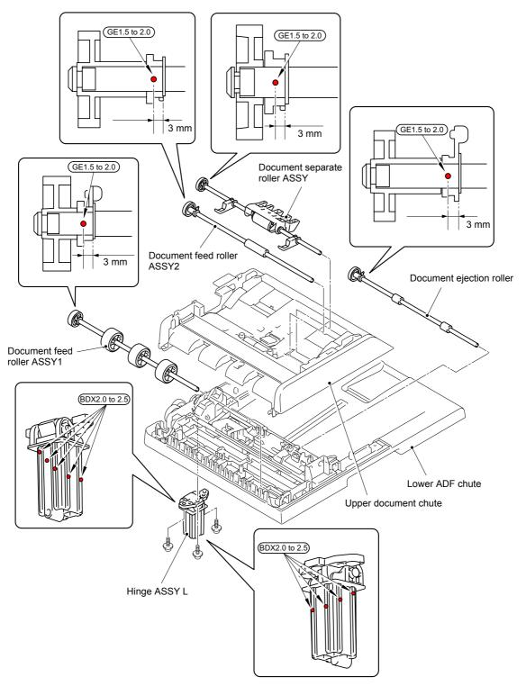
GE1.5 to 2.0: FLOIL GE-676 (1.5 to 2.0 mm dia. ball) BDX2.0 to 2.5: BDX313 (A) (2.0 to 2.5 mm dia. ball)
