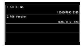
(2) Hold down the blank space at the bottom of the LCD for about 2 seconds. The following screen is displayed on the LCD.
