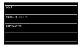
The main firmware version is shown on the second line, and the panel firmware version on the third line.
