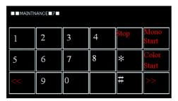
(4) To select one of the maintenance mode functions shown in P5-3, directly enter the function code that you want to use with the ten-key pad.
