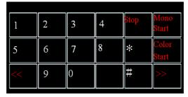
(3) Press the \*, 2, 8, 6, and 4 keys on the LCD in this order. The following screen appears on the LCD and the machine enters the maintenance mode.
