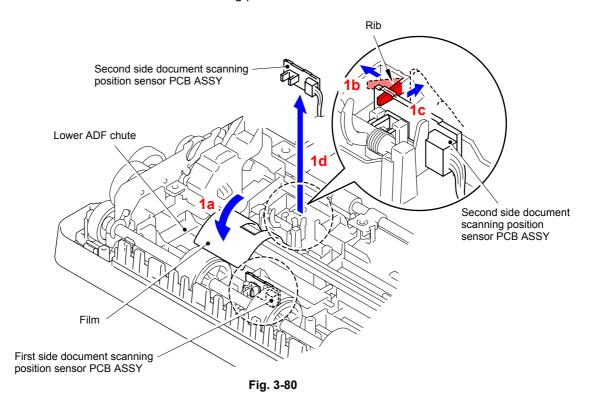
(2) Disconnect the Connector from the Second side document scanning position sensor PCB ASSY.
