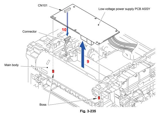
Harness routing: Refer to " 10 Low-voltage Power Supply PCB ASSY"
