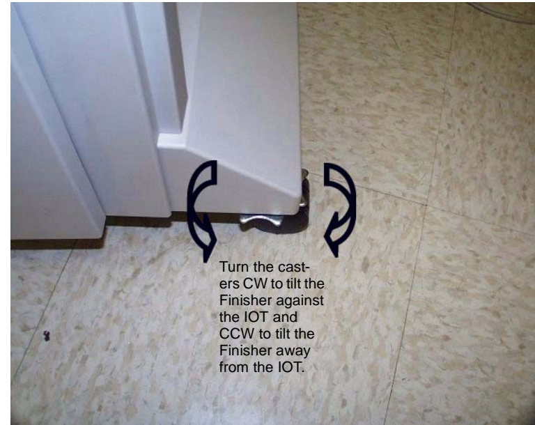
Figure 2 Leveling the Finisher
