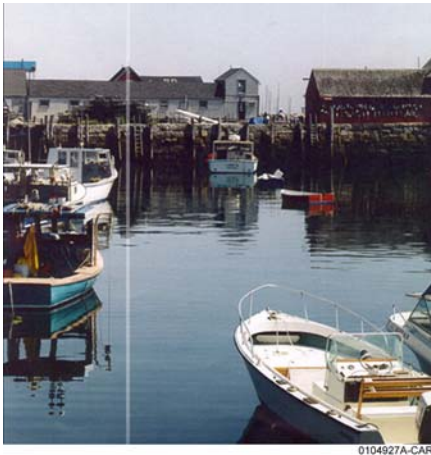
Figure 1 Streak Deletion Defect Sample
