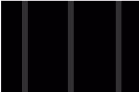
Figure 1 Charging Roll Pitch White Lines (type 1) Defect Sample
