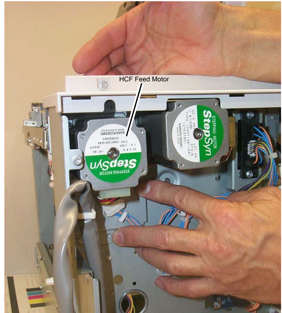
Figure 1 Removing the HCF Feed Motor
