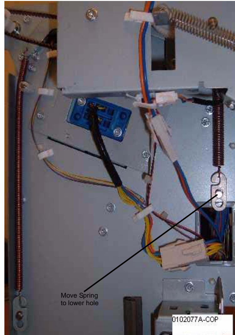
Figure 4 Adjusting the rear Spring tension
