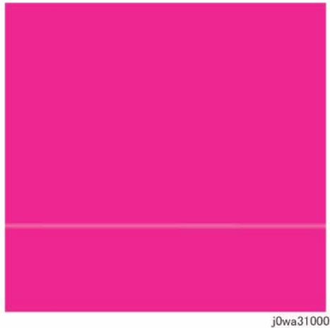
Figure 1 1mm Lines Defect Sample
