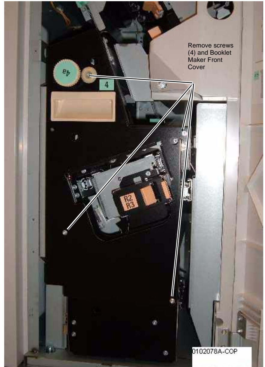
Figure 2 Removing the Booklet Maker Front Cover
