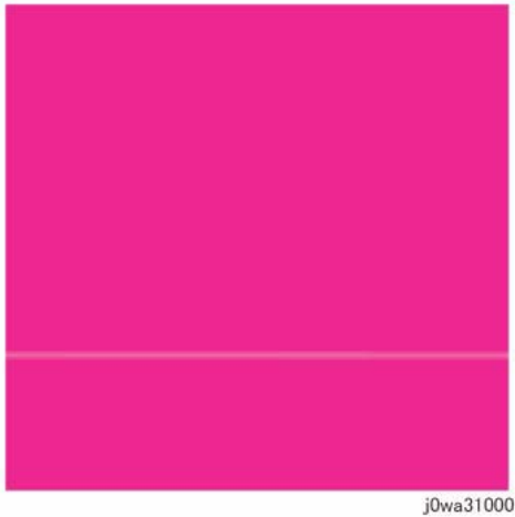
Figure 1 1mm Lines Defect Sample
