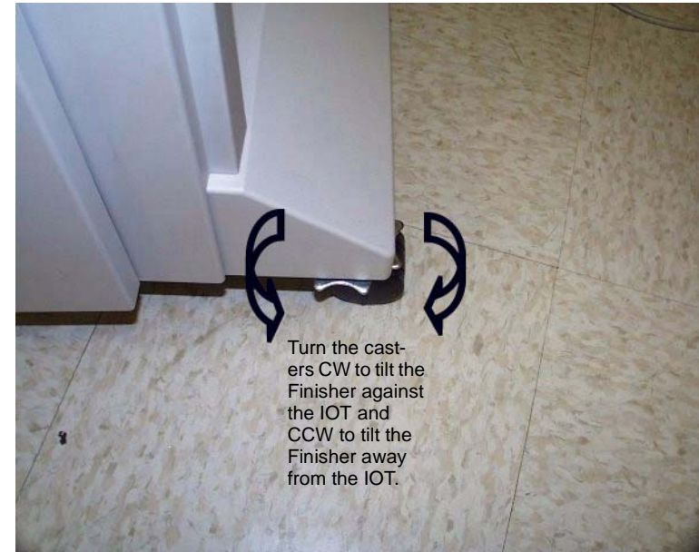
Figure 2 Leveling the Finisher
