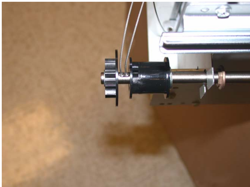
Figure 9 Releasing the Cable ends from the Lift Shaft
