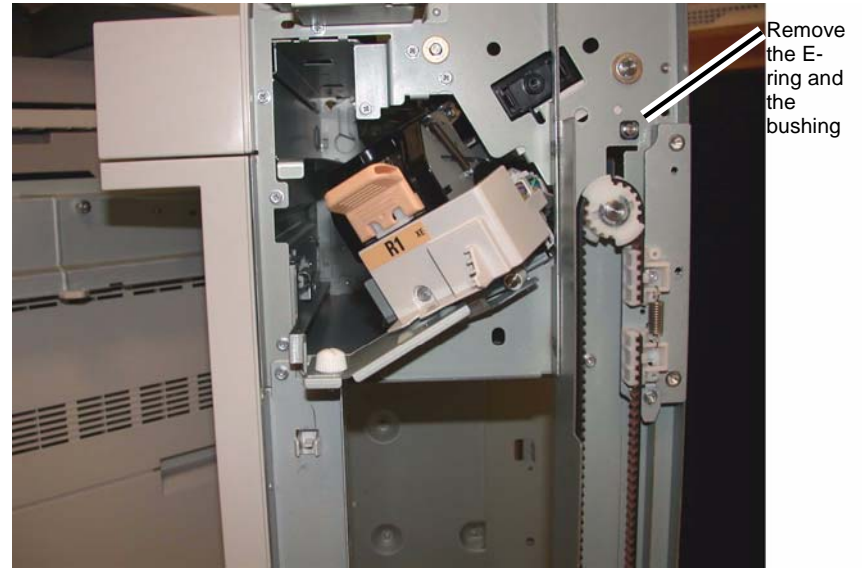
Figure 5 Removing the front E-ring from the Set Clamp Shaft
