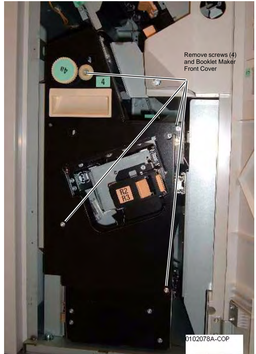
Figure 2 Removing the Booklet Maker Front Cover
