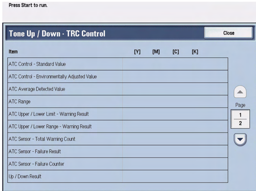
Figure 1 Sample TRC Control Screen 1 of 2
