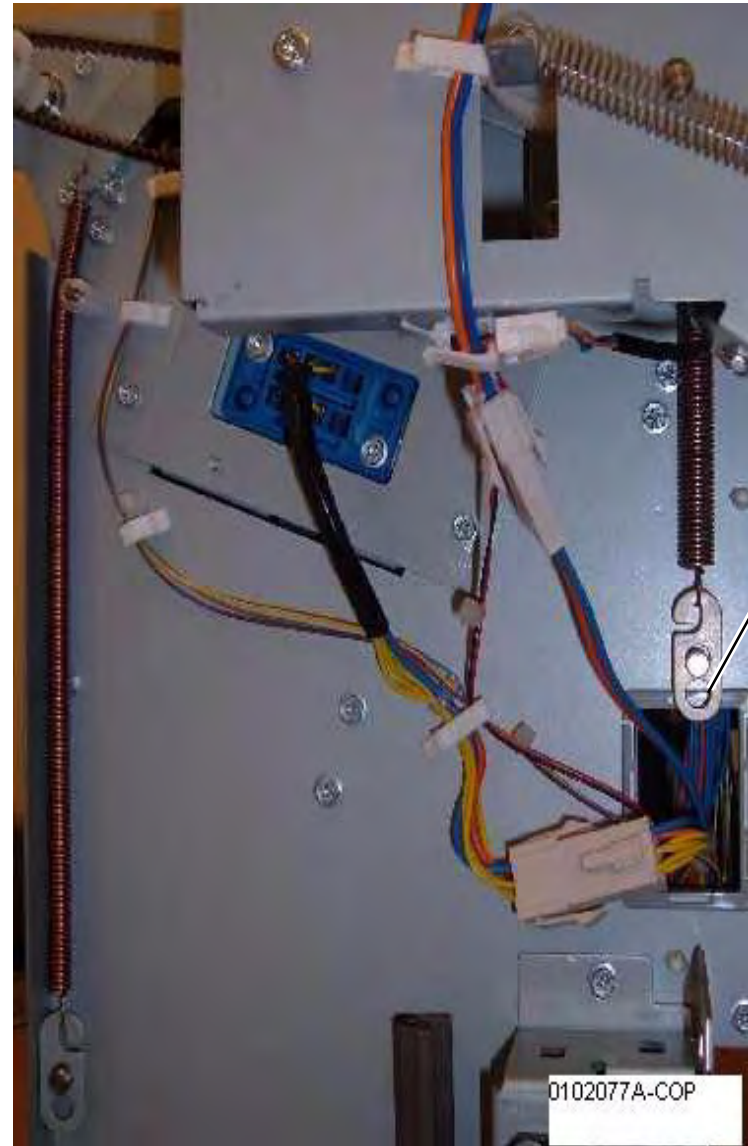
Figure 4 Adjusting the rear Spring tension
