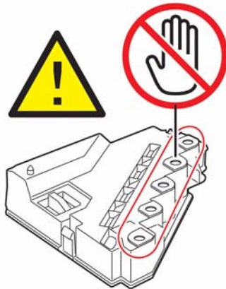
Figure 5 Keep Waste Cartridge Openings Facing Up
