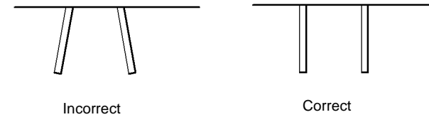
Figure 2 Correct sprung bracket position
