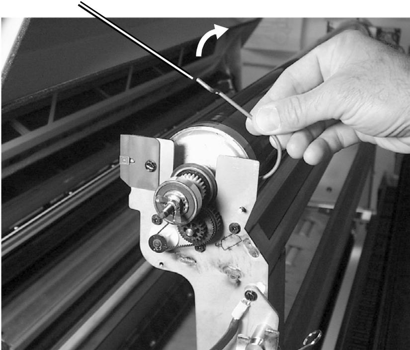
Figure 6 Releasing the Bearing (Left Side) out of the Frame
