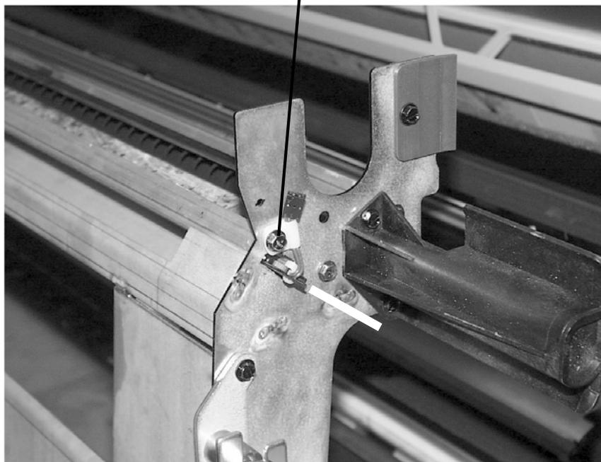
Figure 1 Removing the Erase Bar
