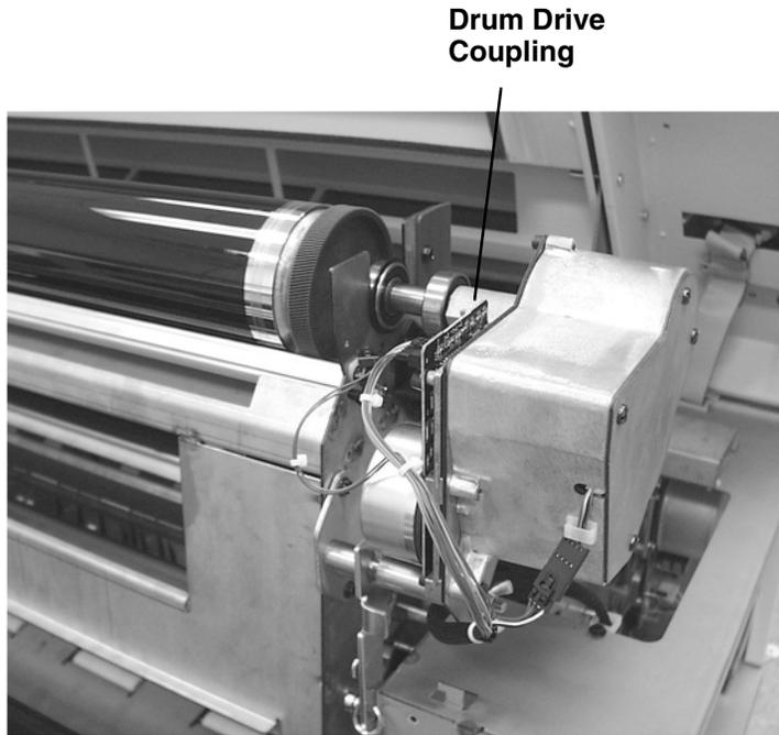
**NOTE:** In the next step, you will need to stop the Drum by hand in order to prevent the Drum from moving (coasting) by the Developer Module and putting a reverse image on the Drum. The Drum Drive Motor is a low torque motor and will stop easily. Place your hand lightly on the Drum Drive Coupling in preparation to stop the Drum then open the interlock.
