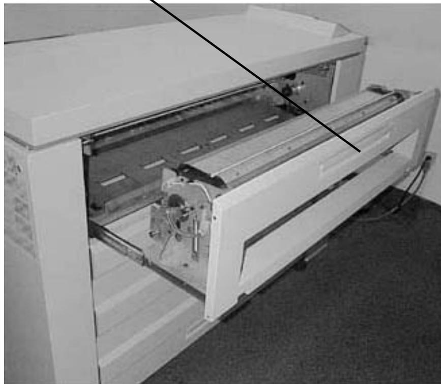
**Figure 1 Accessing the Fuser Module**
