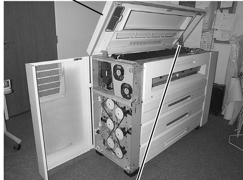
2. Do not release the Top Cover until the latch engages
