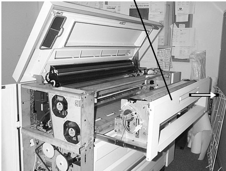
**Figure 2 Partially Extending the Fuser Drawer**
