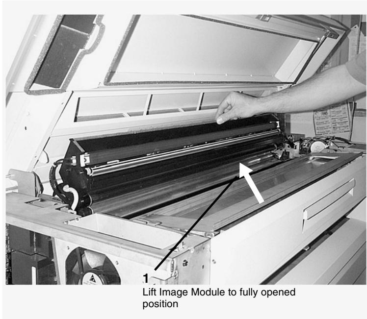
**Figure 1** Lifting the Image Module
