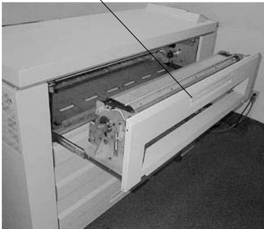
**Figure 1 Accessing the Fuser Module**
