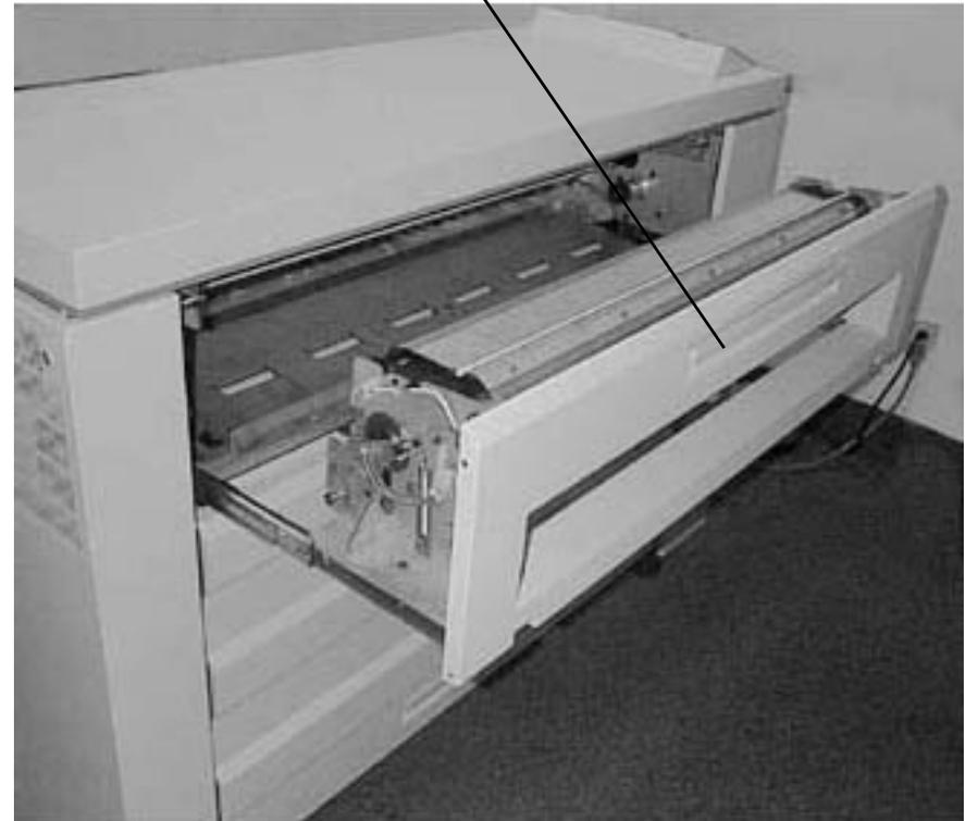
Figure 1 Accessing the Fuser Module
