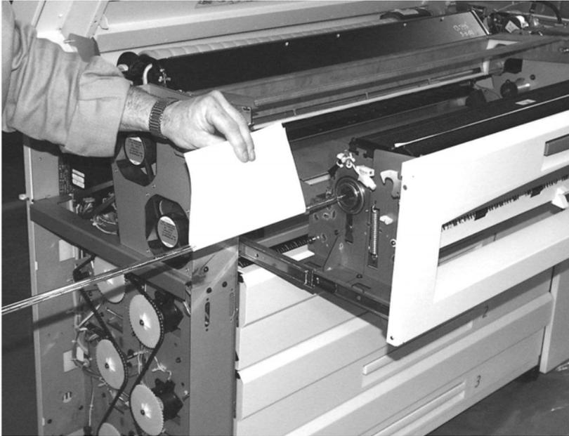
Figure 7 Inserting a Heat Rod into the rear of the fuser
