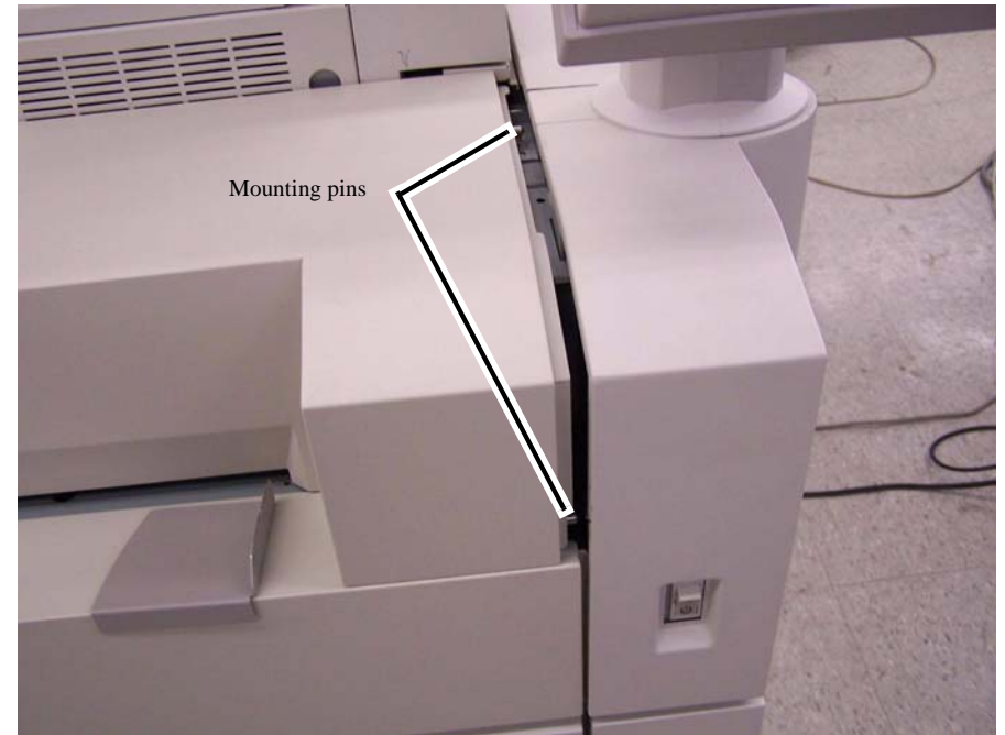
Figure 2 Front Top Cover slid to the left
