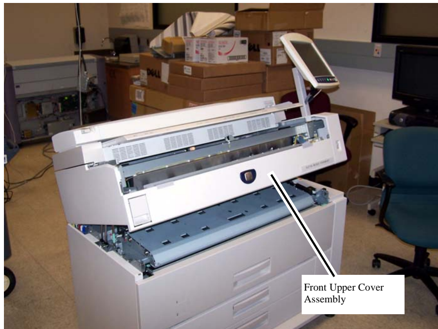
Figure 5 Front Upper Cover Assembly
