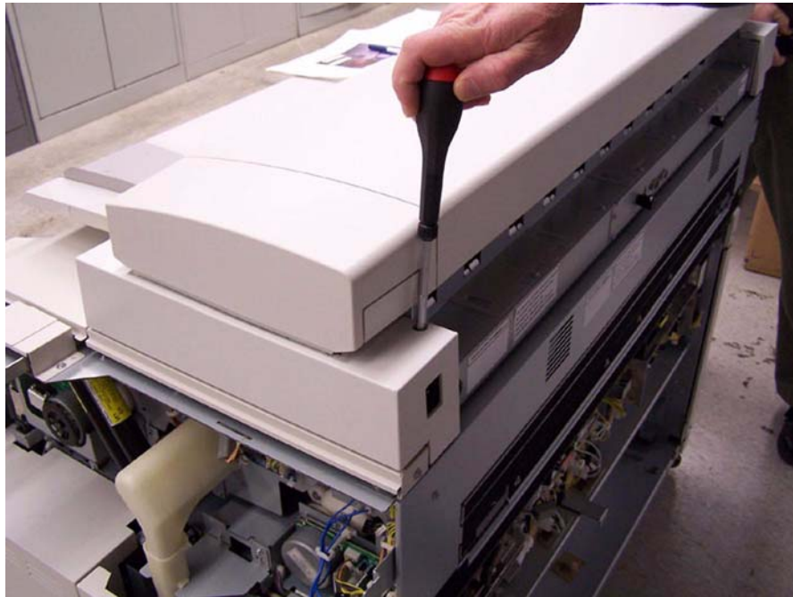
Figure 3 Removing the rear mounting screw
