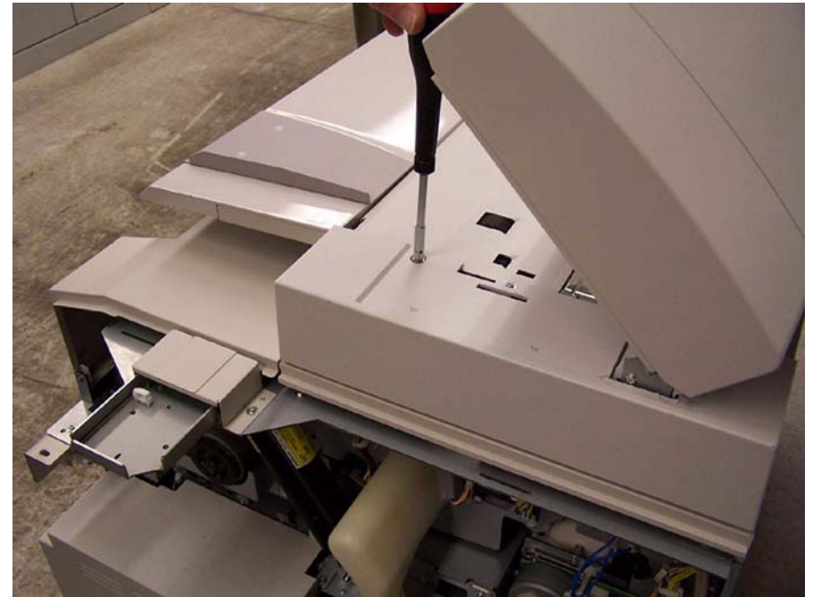
Figure 2 Removing the front mounting screw
