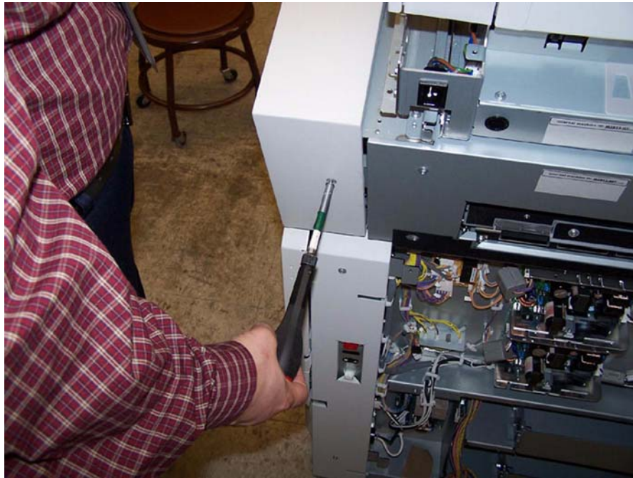
Figure 2 Removing the Right Upper Cover rear mounting screws
