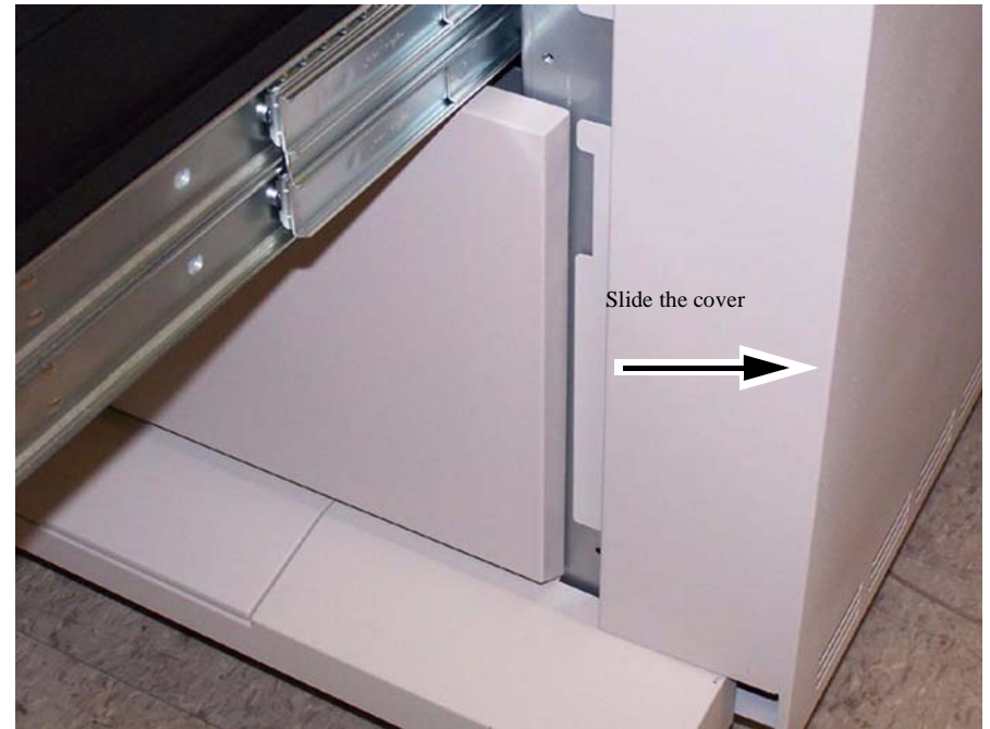
Figure 4 Removing the front of the Right Lower Cover
