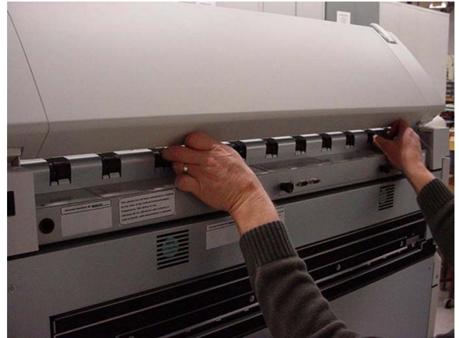
Figure 3 Removing the IIT Lower Baffle
