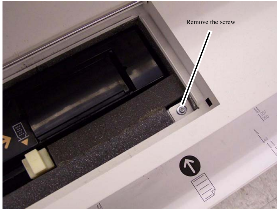
Figure 1 Remove the screw beneath the Toner Cartridge Cover
