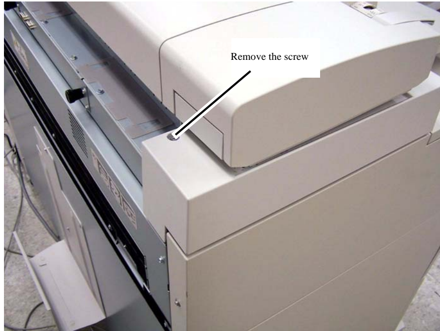
Figure 2 Rear screw location
