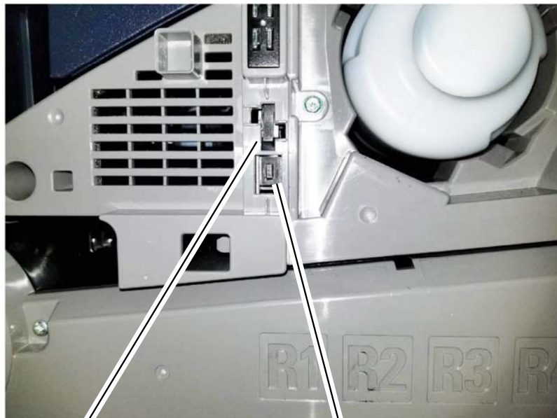
Front cover interlock switch
