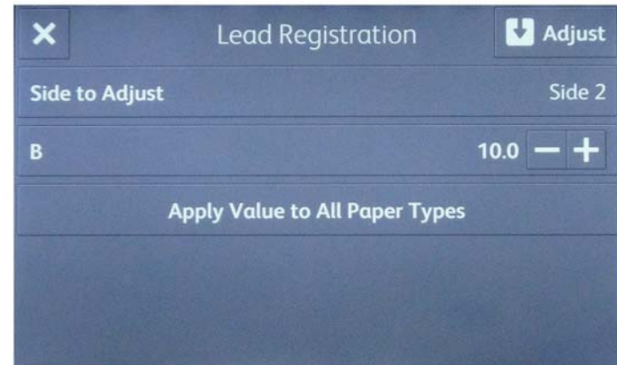
Figure 21 Lead Registration Side 2 input
