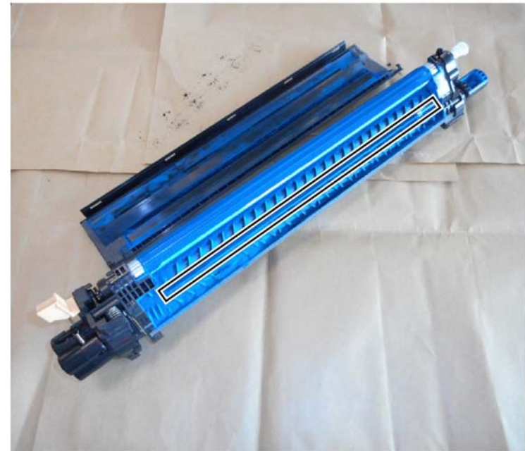
Figure 7 Clean housing area
