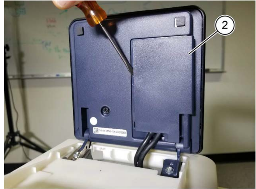
Figure 2 Cable cover removal
