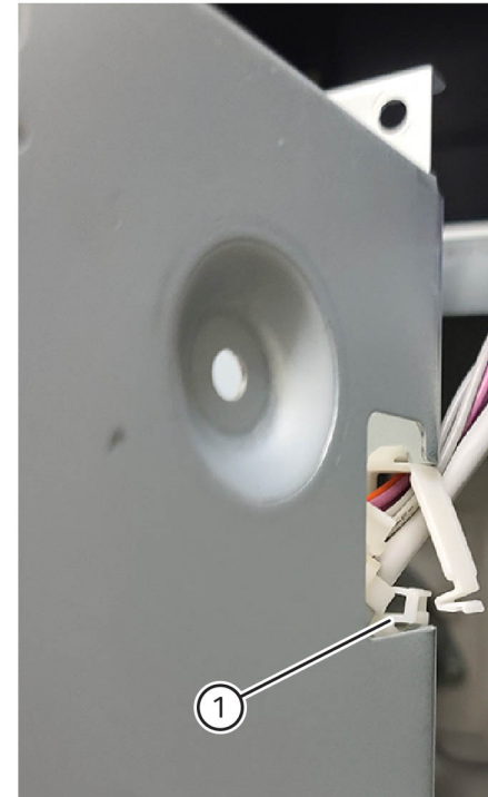
Figure 7 Backside of the chassis harness clamp
