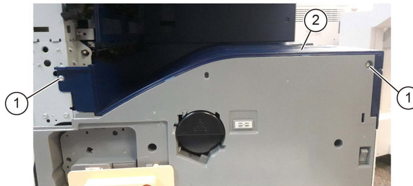
Figure 1 Top cover removal
