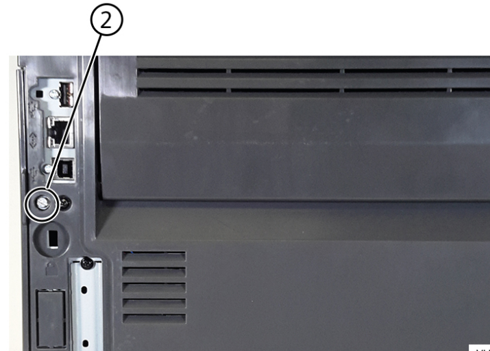
Figure 2 Controller PWB access door screw.
