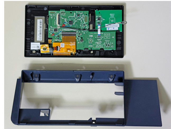
Figure 3 UI control panel and base separated.
