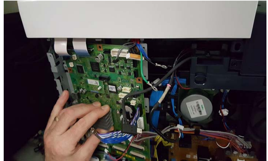
Figure 6 Slide the ESS PWB from the Right Side of the ESS Frame
