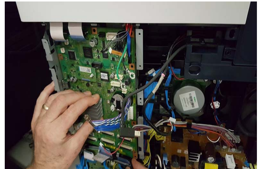
Figure 5 Lift the Bottom Right Corner from the ESS Frame
