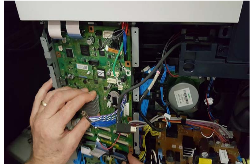
Figure 4 Lift the Bottom Right Corner from the ESS Frame
