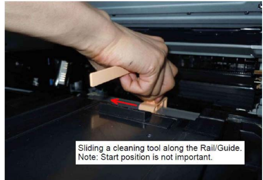
Figure 4 Cleaning wand positioning
