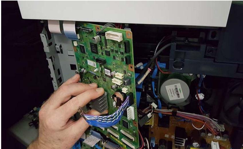
Figure 6 Remove the ESS PWB from the ESS Frame
