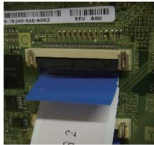
Figure 6 FFC cable installation
