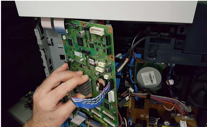
Figure 7 Remove the ESS PWB from the ESS Frame
