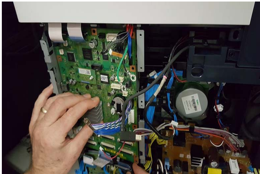
Figure 5 Lift the Bottom Right Corner from the ESS Frame
