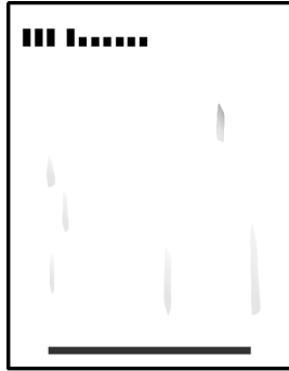
Figure 1 Example of Smudged or Smeared Output
