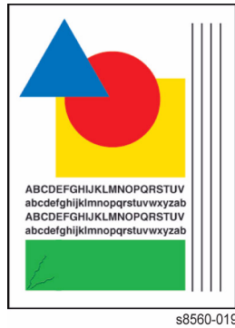
Figure 1 Example of Wrinkled Output
