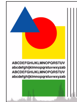
Figure 1 Example of Oil Streaks on Output
