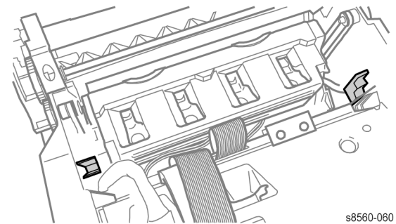
Figure 9 Printhead Cradle Notch Location
