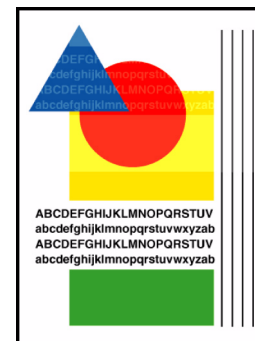
Figure 1 Example of Ghosting on Output
