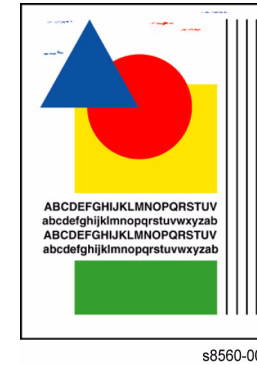
Figure 1 Example of Latent Image on Output
