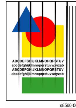
Figure 1 Example of Streaks and Lines on Output
