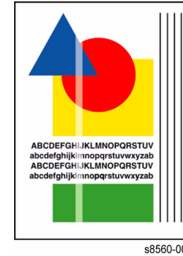
Figure 1 Example of Scratches on Output
