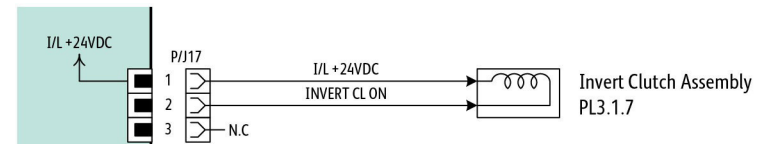
Figure 1 Example Clutch Wiring Diagram
