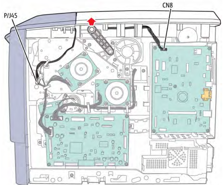
Figure 1 Disconnect the Control Panel and Top Door linkage
