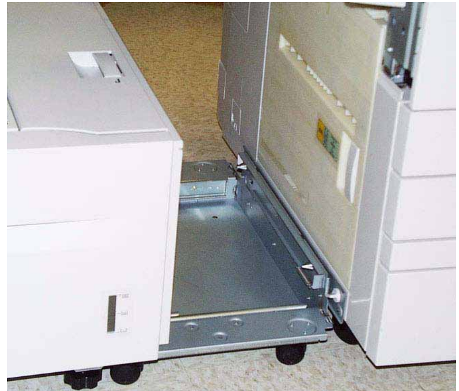
Figure 1 Exposing the docking base
