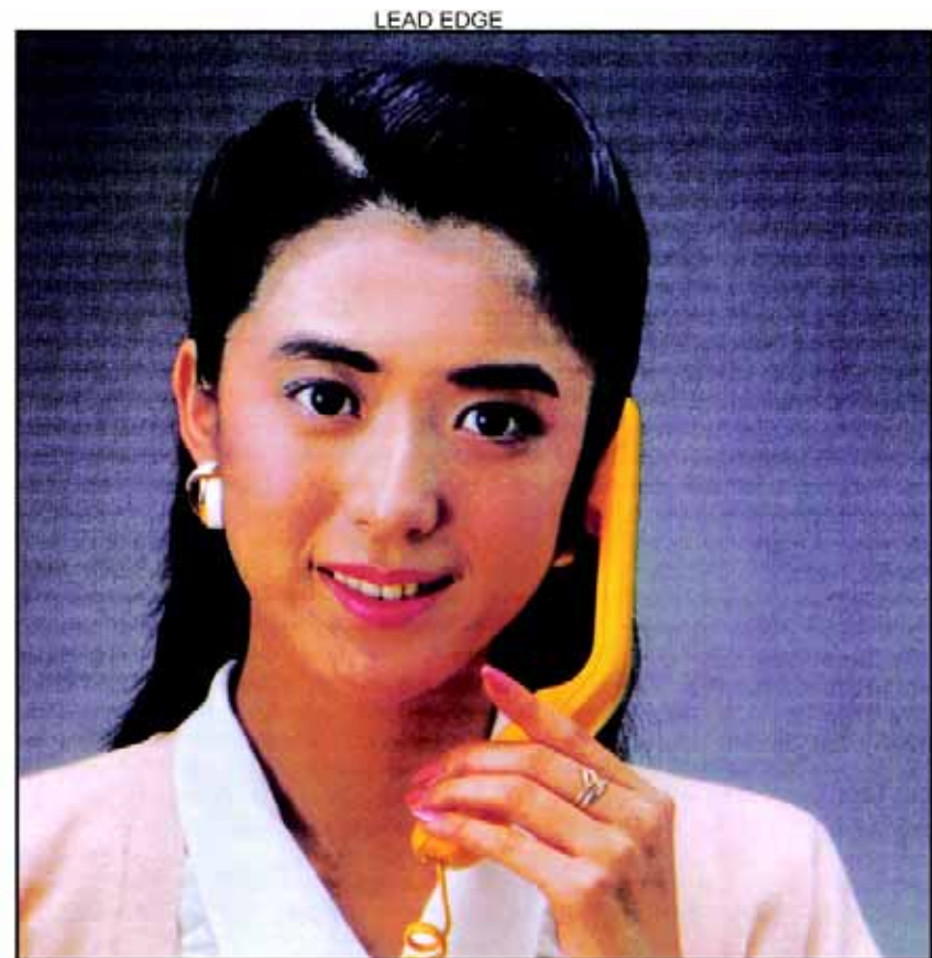
Figure 1 High Freq. Bands Defect Sample
