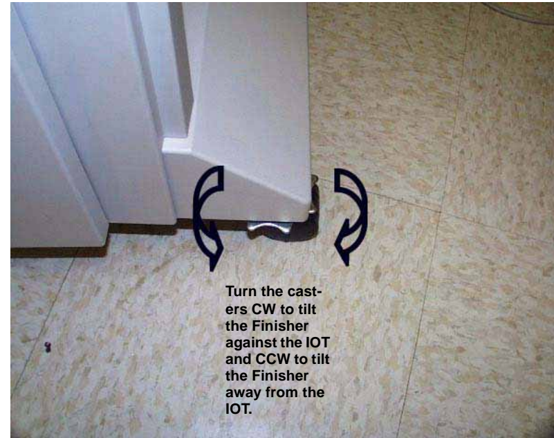
Figure 2 Adjusting Finisher Level
