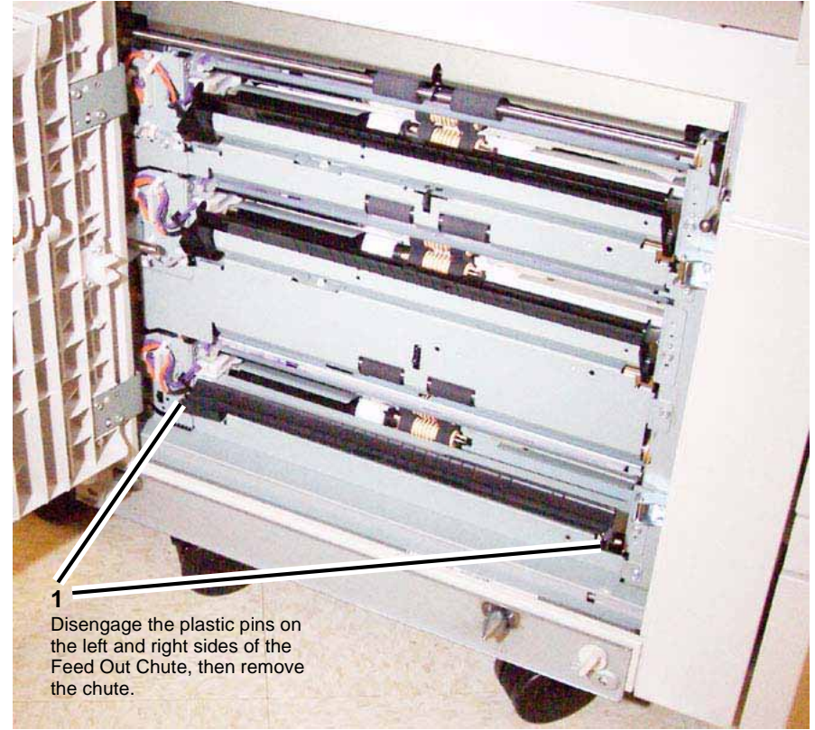
Figure 3 Removing the Feed Out Chute
