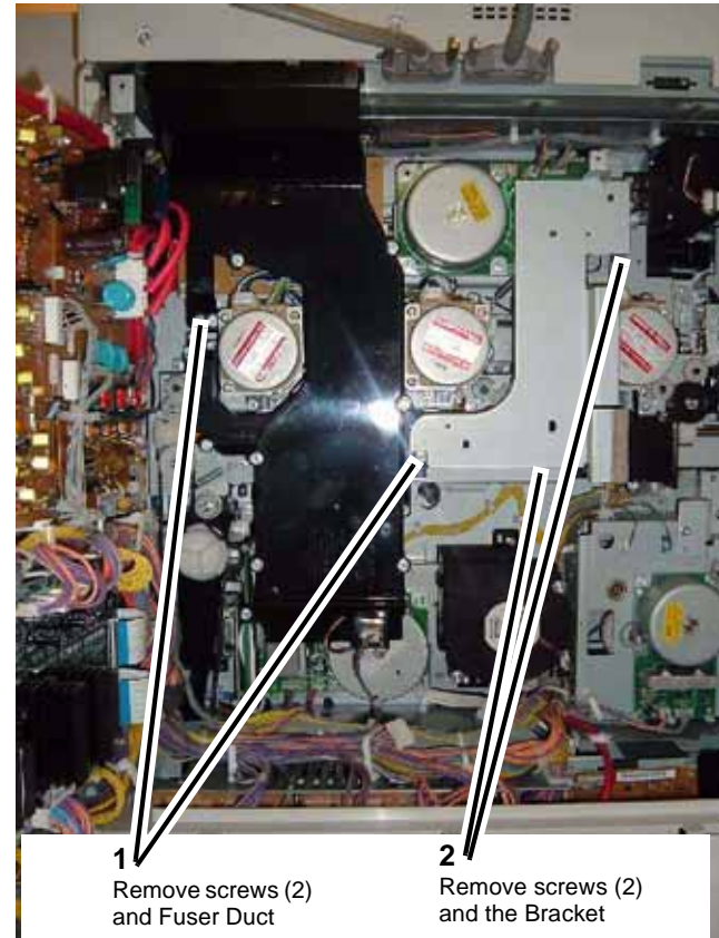
Figure 3 Removing Fuser Duct and Bracket
