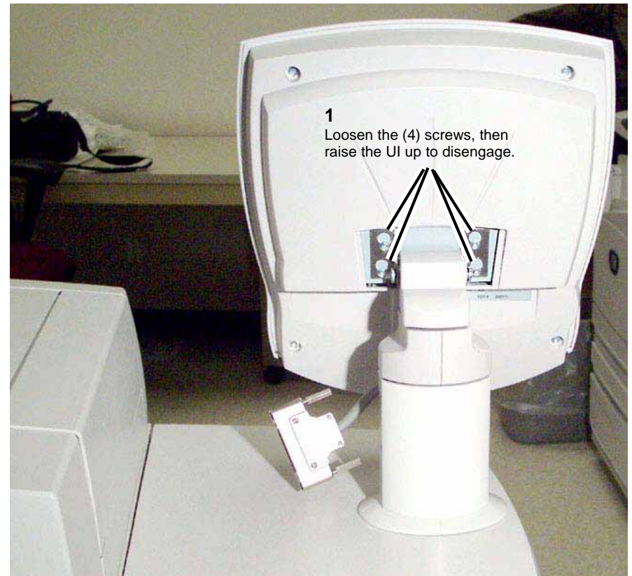
Figure 1 Removing the UI from the Tilt Swivel brackets
