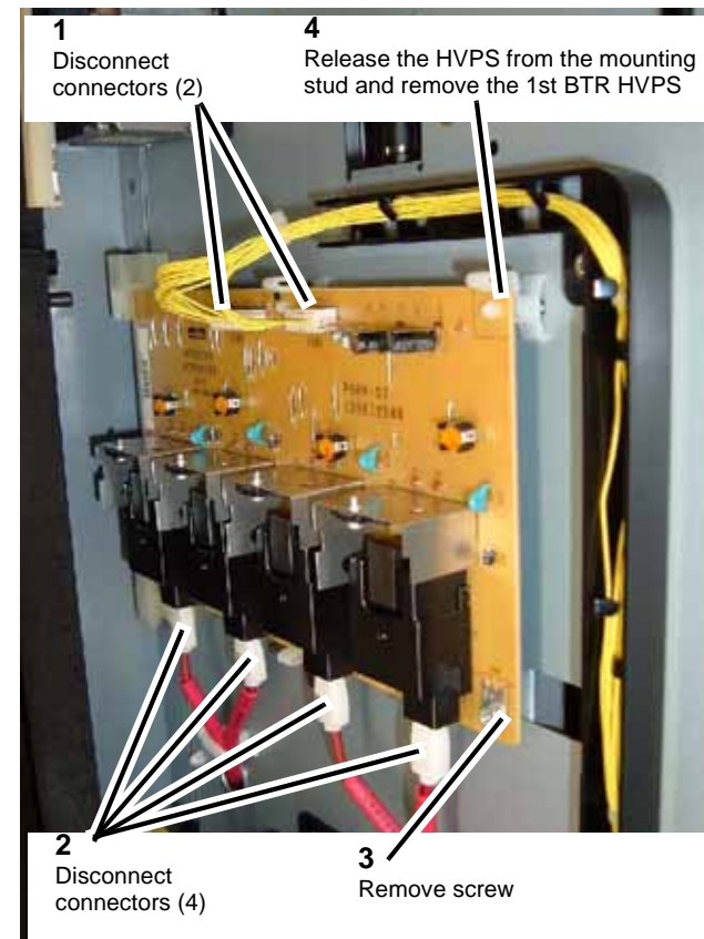
Figure 1 Removing the 1st BTR HVPS
