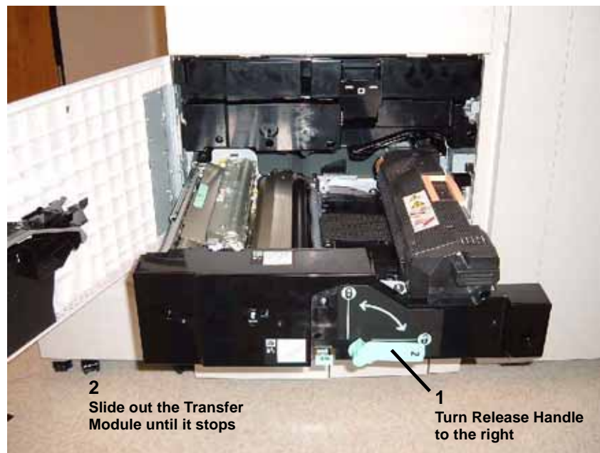
Figure 1 Opening the Transfer Module
