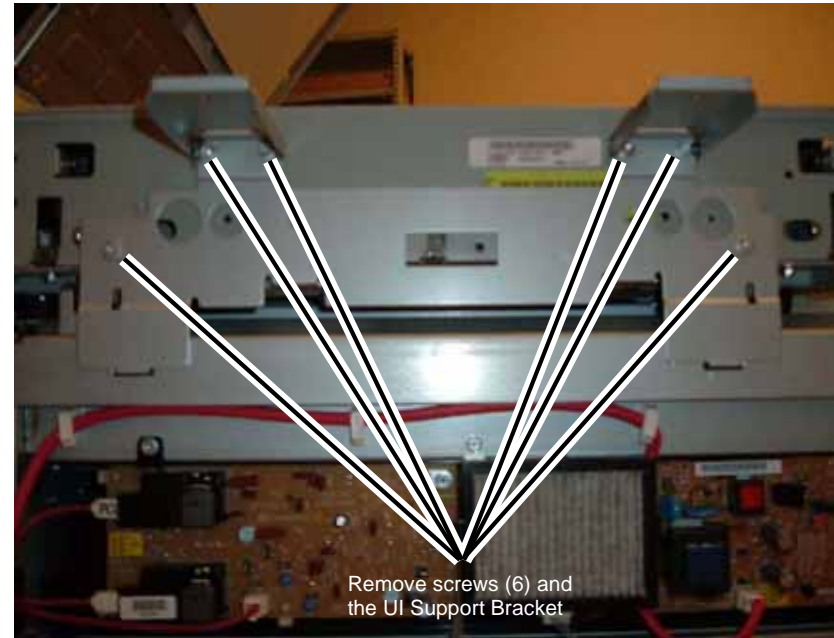
Figure 3 Removing the UI Support Bracket
