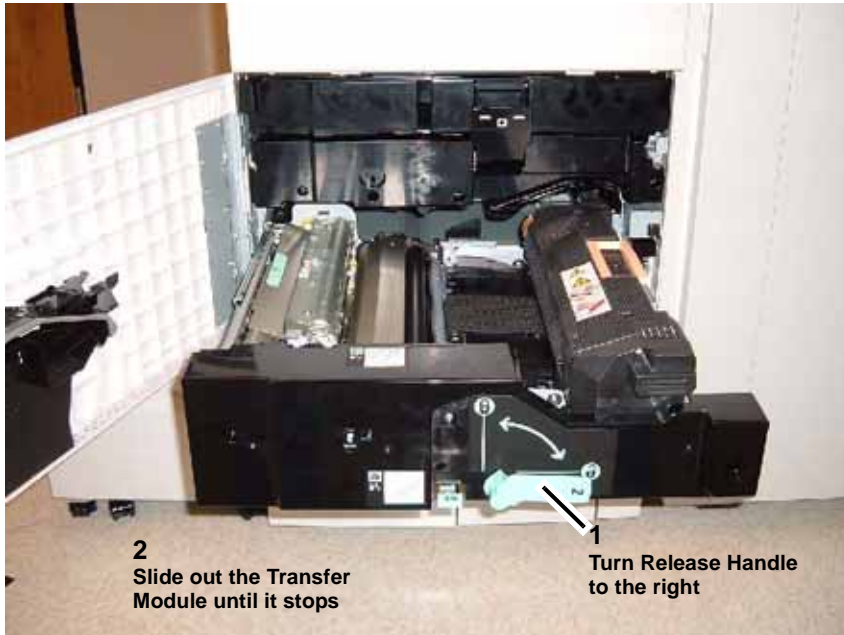
Figure 1 Opening the Transfer Module
