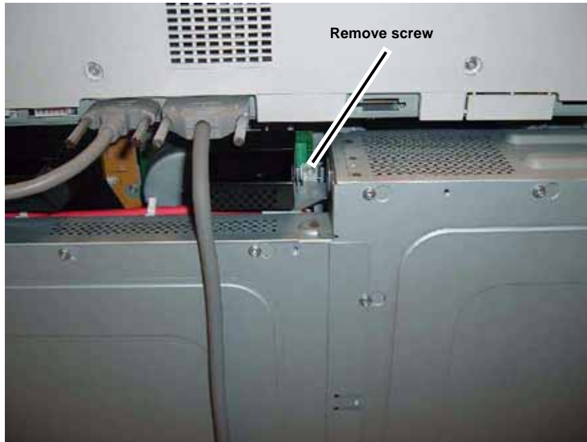
Figure 3 Removing screw securing the Chassis Assembly to the frame
