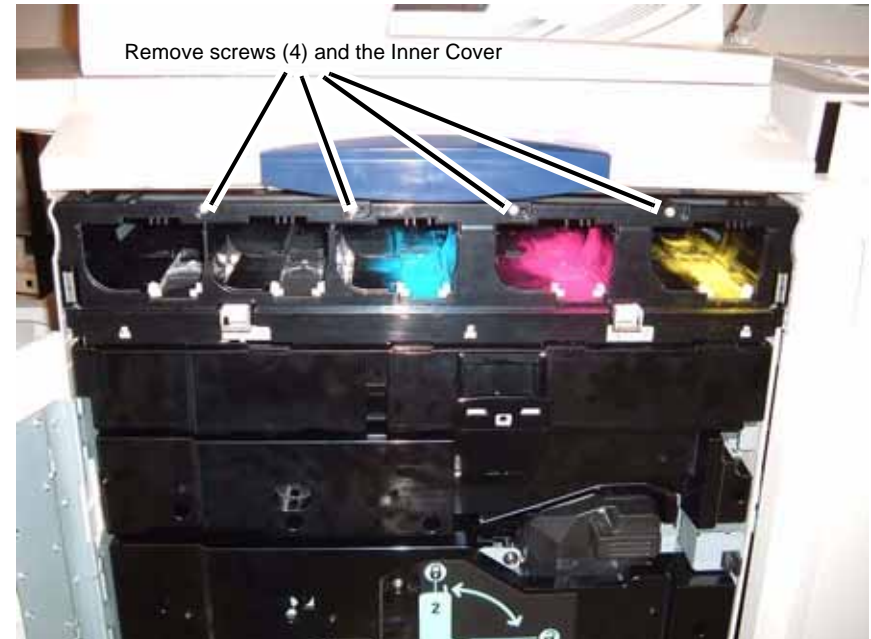
Figure 2 Removing the Inner Cover
