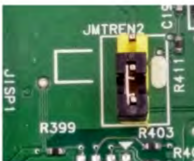
Interlock bypass enabled
