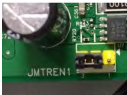
Interlock bypass disabled (default)
