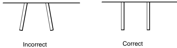
Figure 2 Correct spring bracket position.
