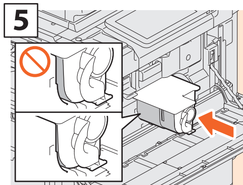
Insert the new toner cartridge until its front surface aligns to the left side wall.
