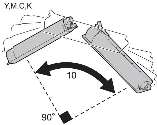
2) Turn the toner cartridge as shown in the figure and pull out the seal.
