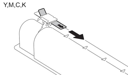
3) Install the corresponding color of toner cartridge in the developer unit.
