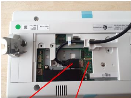
CABLE: OPERATION SUB-UNIT:USB3.0
