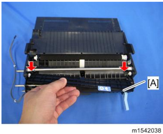
17. Remove the Registration roller (follower) [A] as shown below (spring x 2, plastic parts x 2).
