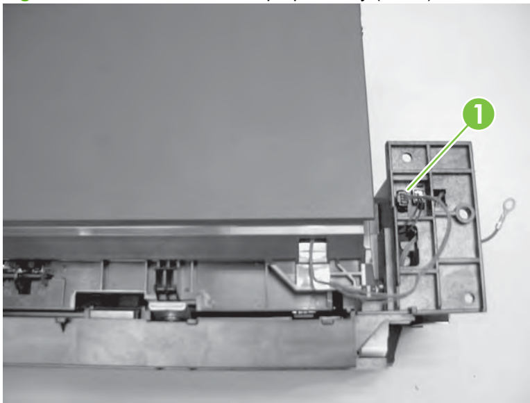
Figure 6-146 Remove the multipurpose tray (4 of 5)
