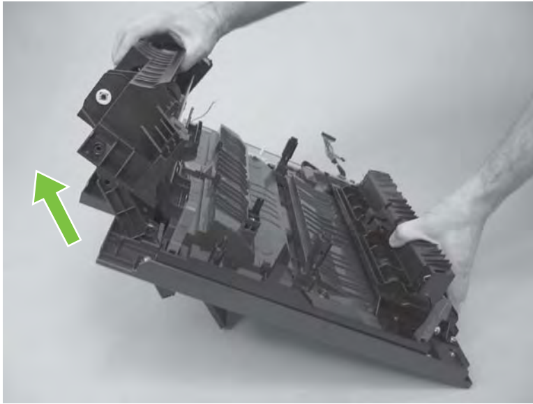
Figure 6-145 Remove the multipurpose tray (3 of 5)
