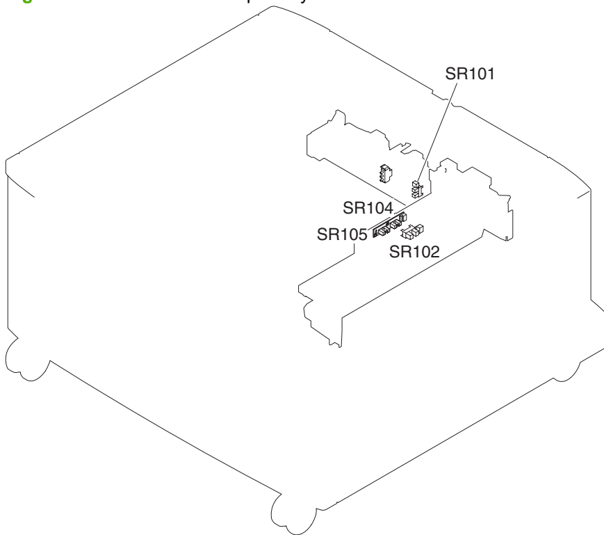
Figure 7-35 1 x 500-sheet input-tray sensor locations
