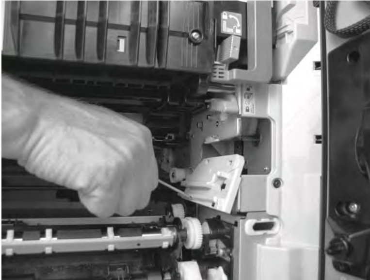
Figure 6-3 Remove the secondary transfer unit (1 of 9)
