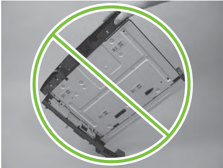
Figure 8-101 Incorrect placement of the IPTU (2 of 2)
