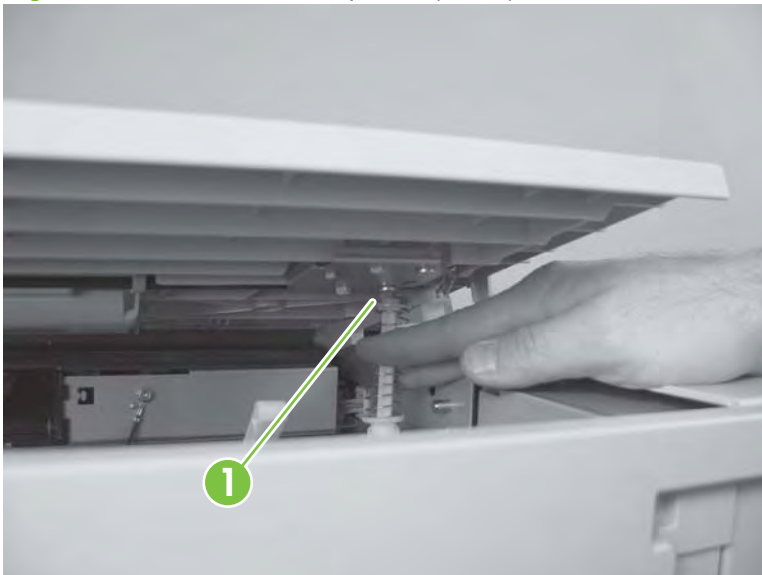
Figure 8-147 Remove the top door (2 of 3)
