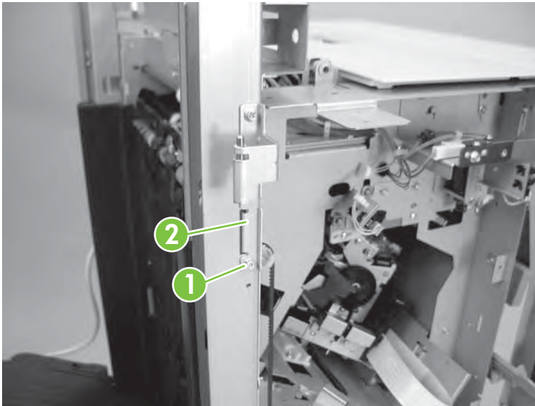
Figure 8-197 Remove output-bin 2 (1 of 3)
