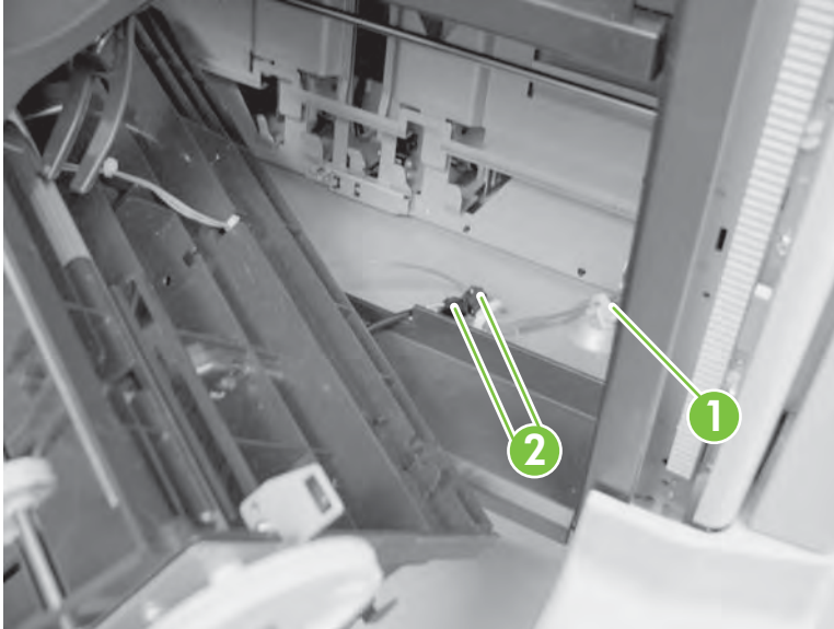
Figure 8-206 Remove the saddle delivery output bin (3 of 3)
