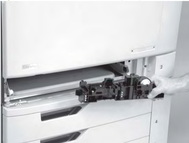
Figure 6-31 Remove the lifter drive unit (2 of 2)
