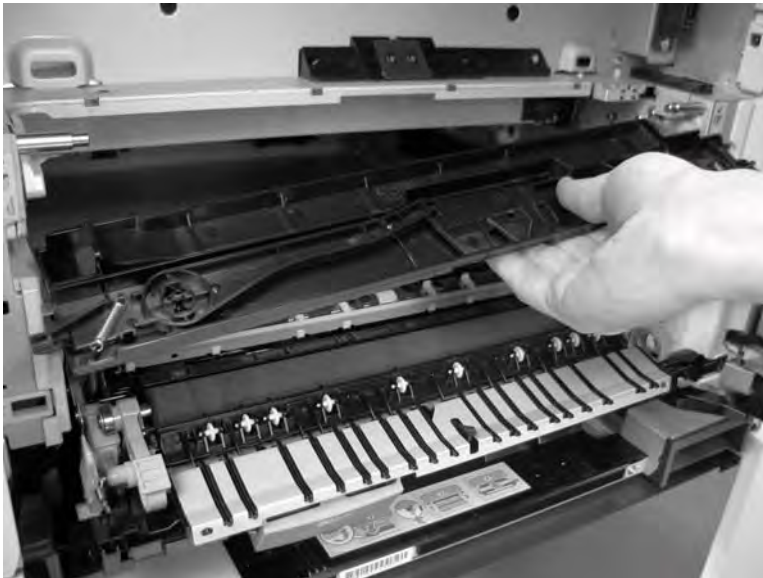
Figure 6-153 Remove the ITB duct (2 of 2)
