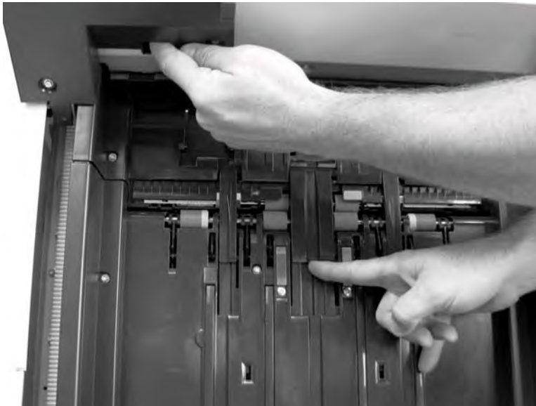
Figure 8-199 Remove output-bin 2 (3 of 3)
