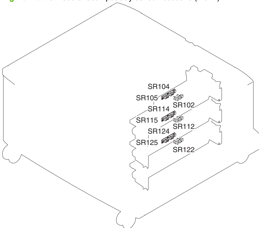
Figure 7-36 3 x 500-sheet input-tray sensor locations (1 of 2)
