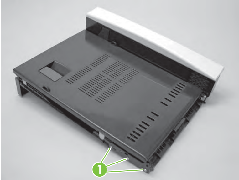
Figure 8-108 Remove upper-guide assembly (1 of 2)
