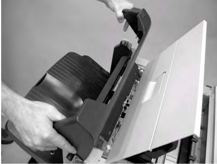
Figure 8-144 Remove the left-upper cover (2 of 3)
