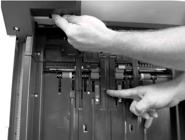
Figure 8-196 Remove output-bin 1 (3 of 3)
