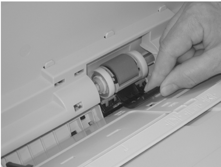
Figure 2-11 Remove the separation pad (Tray 1) (4 of 4)
