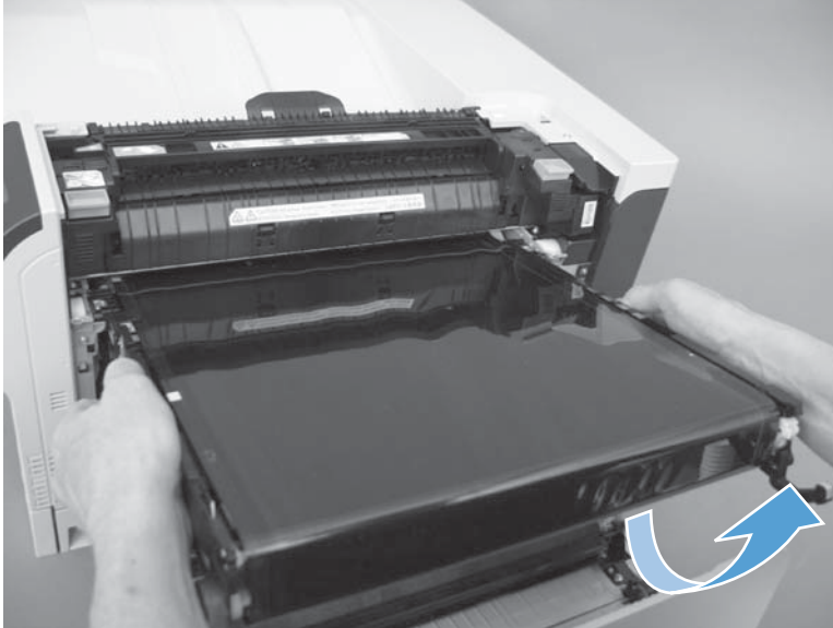
Figure 2-18 Remove the intermediate transfer belt (3 of 3)
