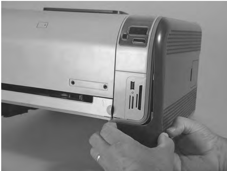
Figure 6-13 Remove the right cover (2 of 4)
