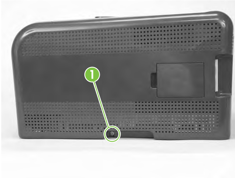
Figure 6-12 Remove the right cover (1 of 4)
