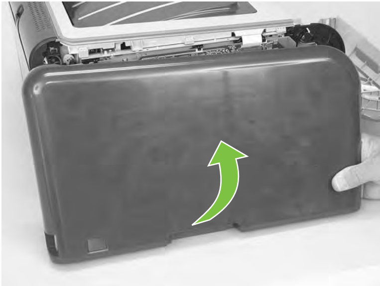
Figure 6-19 Remove the left cover (4 of 4)
