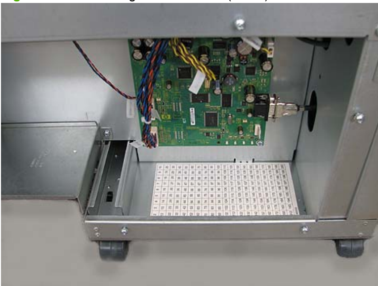
Figure 4-7 Retrofit tag label locations (5 of 7)
