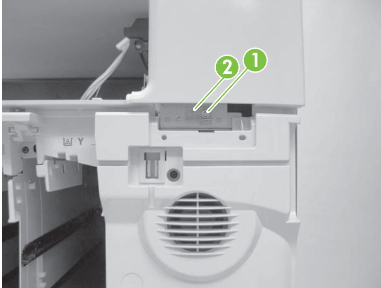
Figure 6-154 Remove optical scanner (2 of 7)
