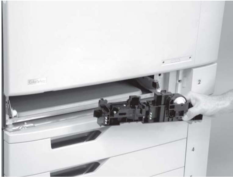
Figure 6-29 Remove the lifter-drive unit (2 of 2)
