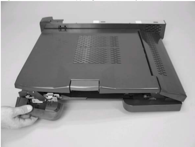
Figure 8-103 Remove upper guide assembly (2 of 5)
