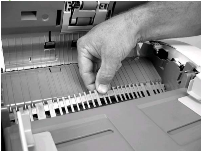
Figure 6-217 Remove the ADF diverter (1 of 2)
