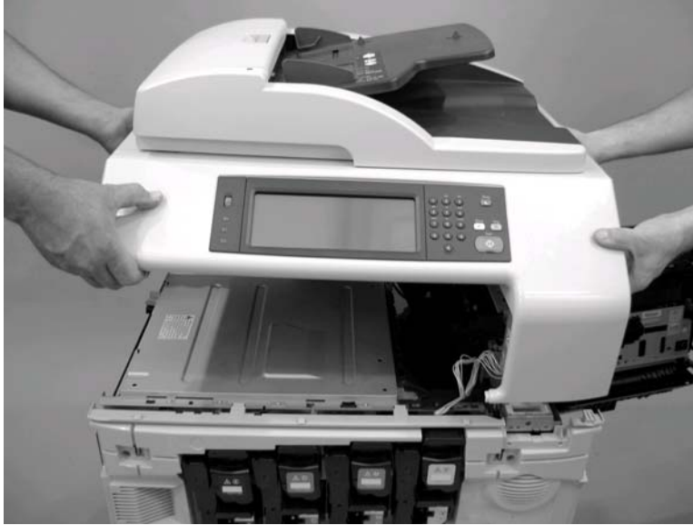
Figure 6-158 Remove optical scanner (6 of 7)
