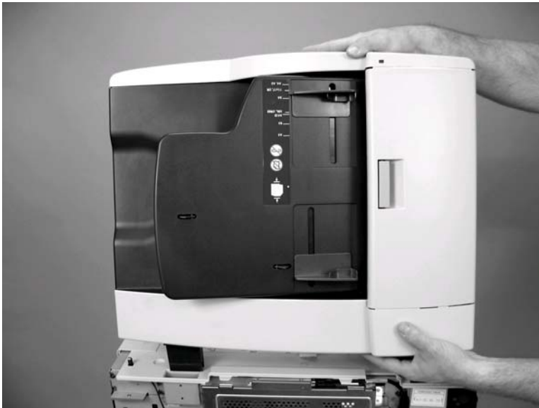
Figure 6-210 Remove the ADF assembly (4 of 4)
