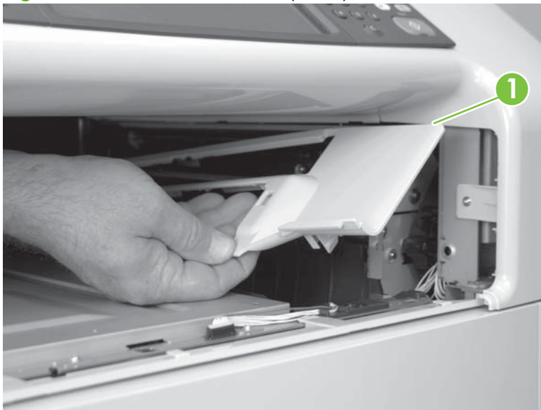
Figure 6-85 Remove inner cover (4 of 4)
