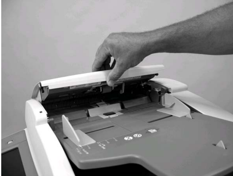
Figure 6-213 Remove the ADF separation floor assembly (1 of 4)
