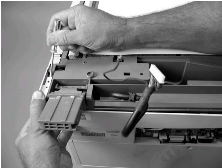
Figure 6-239 Remove the ADF rear end cover (4 of 5)
