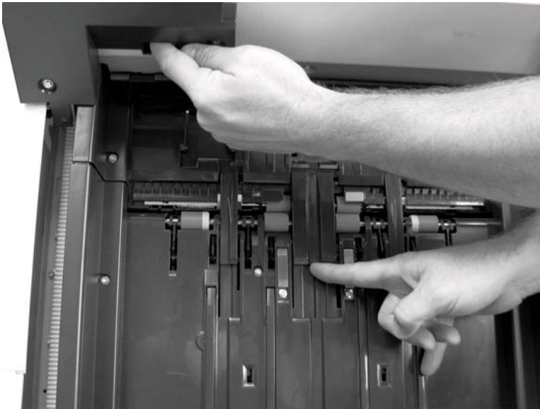
Figure 8-202 Remove output-bin 2 (3 of 3)
