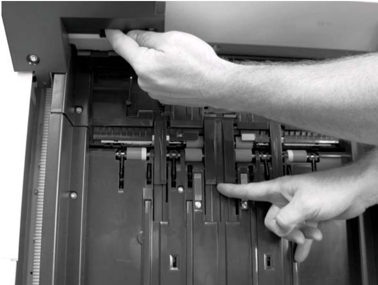
Figure 8-199 Remove output-bin 1 (3 of 3)
