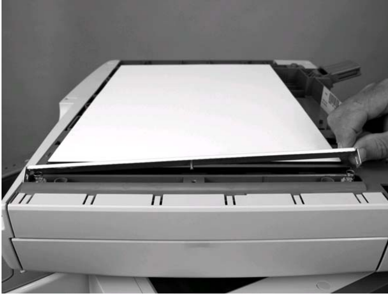
Figure 6-225 Remove the ADF float assembly (3 of 5)
