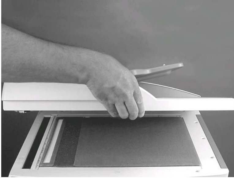
Figure 6-230 Remove the ADF white backing (3 of 4)
