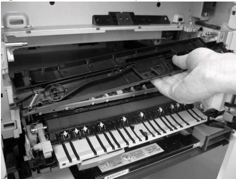
Figure 6-125 Remove the ITB duct (2 of 2)
