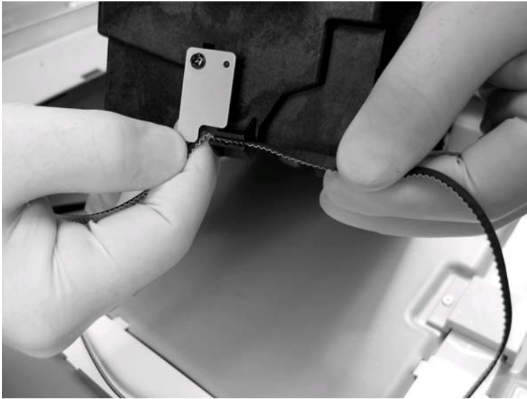
Figure 6-178 Remove carriage unit (6 of 8)
