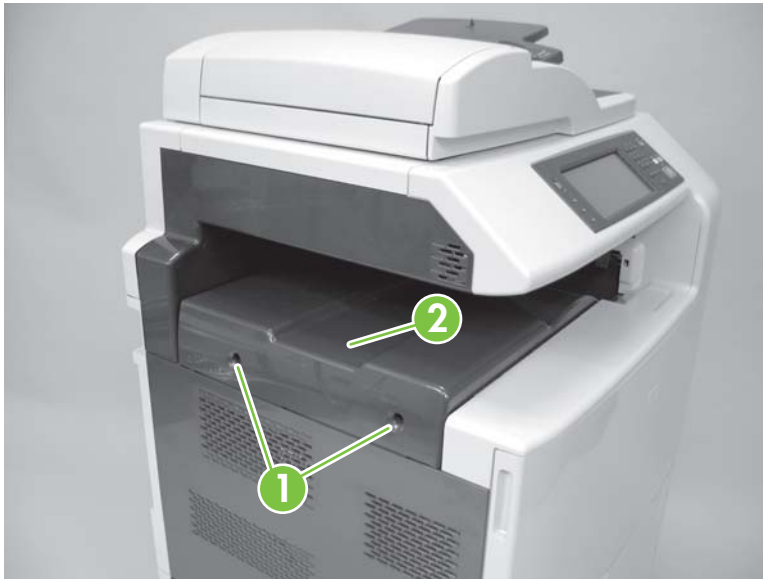
Figure 6-34 Remove face-down output bin
