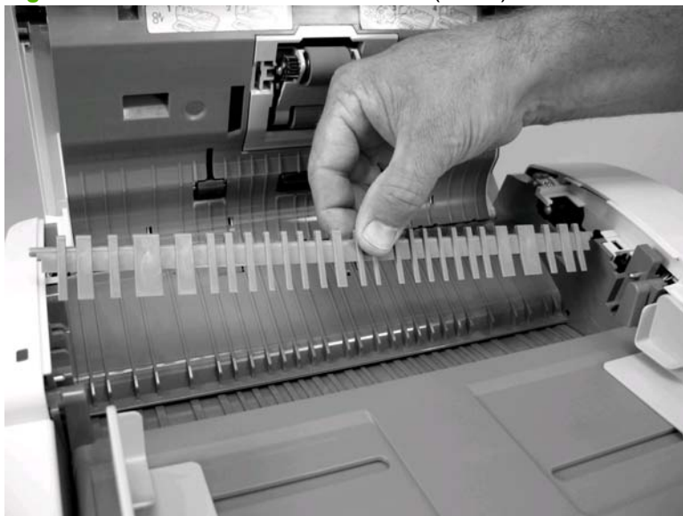
Figure 6-218 Remove the ADF diverter (2 of 2)
