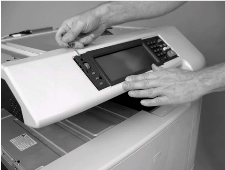
Figure 6-163 Remove control panel (2 of 3)
