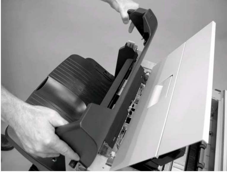
Figure 8-147 Remove the left-upper cover (2 of 3)
