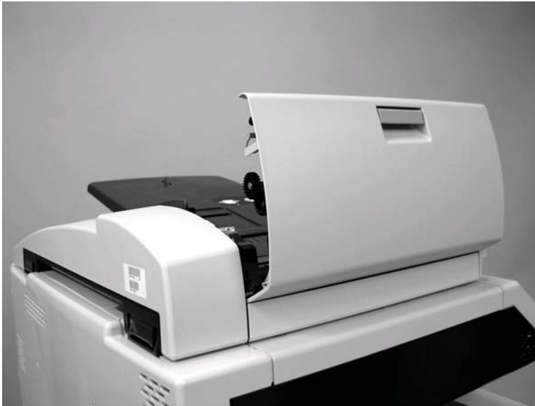
Figure 6-219 Remove the ADF jam cover (1 of 3)
