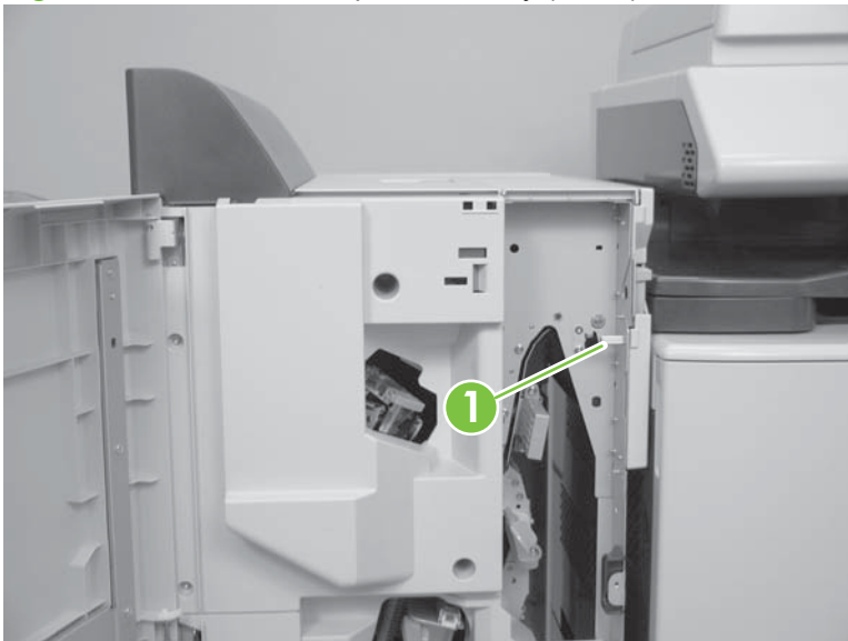
Figure 8-132 Remove output accessory (2 of 5)
