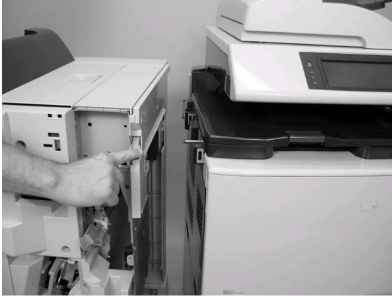
Figure 8-133 Remove output accessory (3 of 5)
