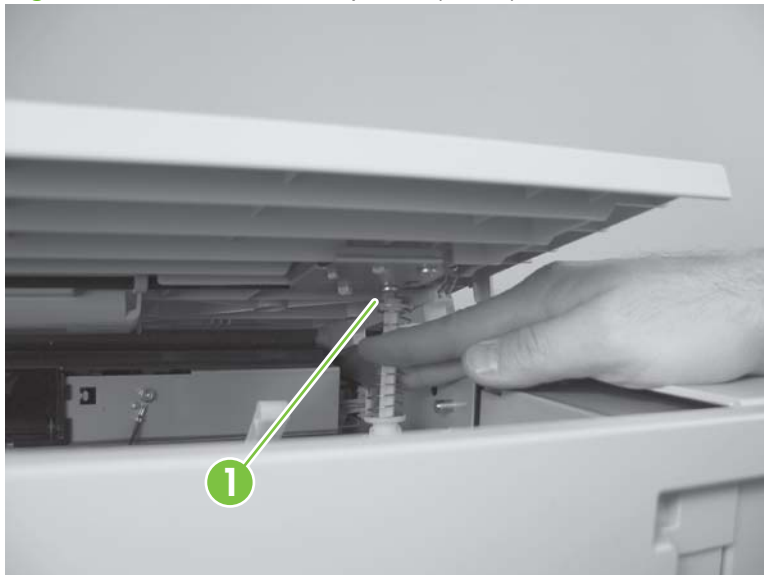
Figure 8-150 Remove the top door (2 of 3)
