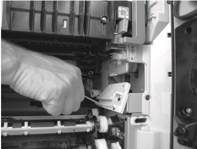
Figure 6-2 Remove the secondary transfer unit (1 of 9)
