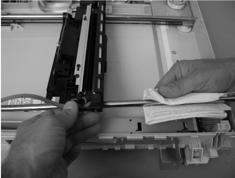
Figure 2-129 Remove the S-PBA-TYUKEI (interconnect board) and S-SNS-EY3A1061-2 (size sensor) (2 of 4)
