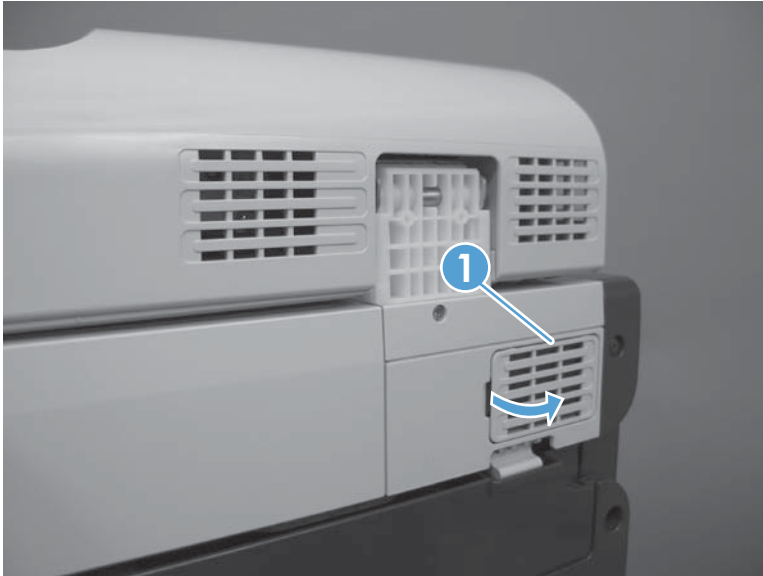
Figure 2-107 Remove the scanner filter (1 of 2)
