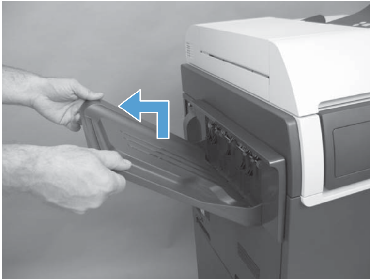
Figure 2-40 Remove the standard output bin
