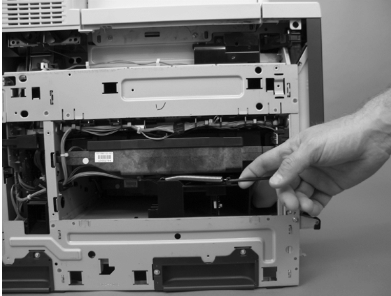
Figure 2-185 Remove the cartridge fan and environmental sensor (2 of 7)
