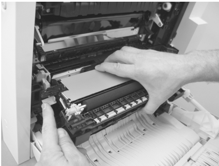
Figure 2-157 Reinstall the secondary transfer assembly
