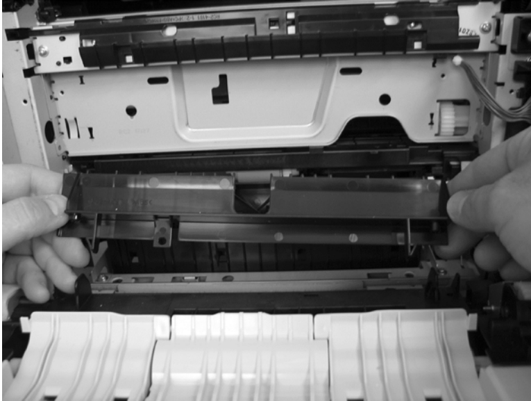
Figure 2-251 Remove the tray-pickup assembly (7 of 11)
