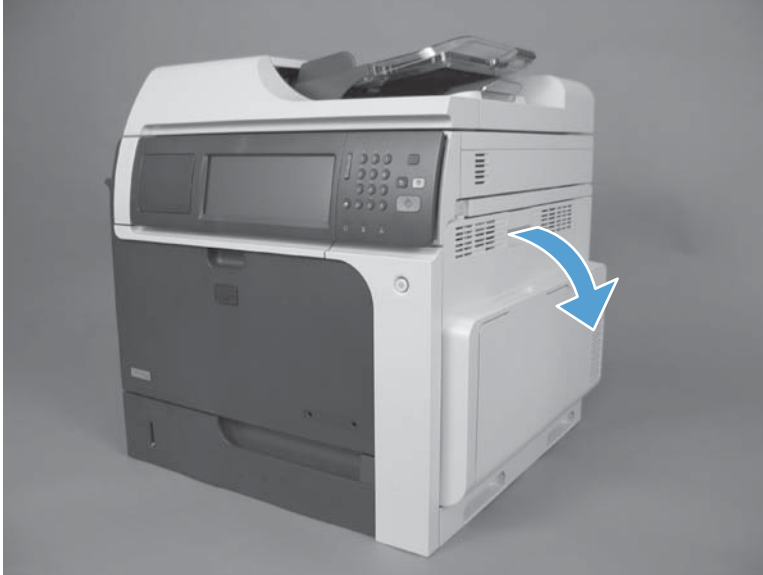
Figure 2-151 Remove the cassette feed guide (1 of 3)
