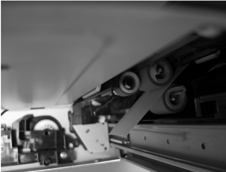
Figure 3-32 Test the Tray 3 feed sensor
