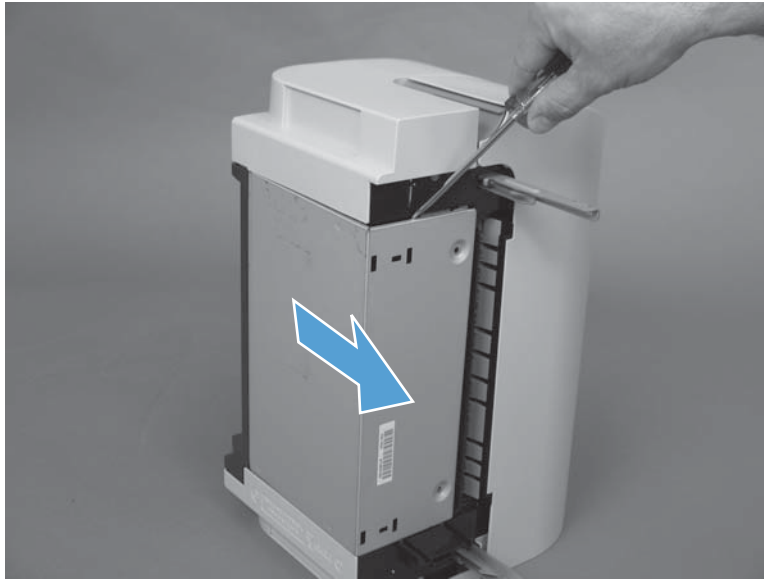
Figure 2-354 Remove the output bin 3 drive assembly (2 of 3)
