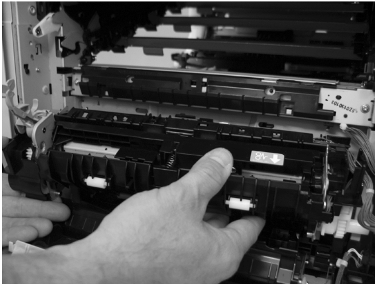
Figure 2-178 Remove the registration assembly (8 of 8)
