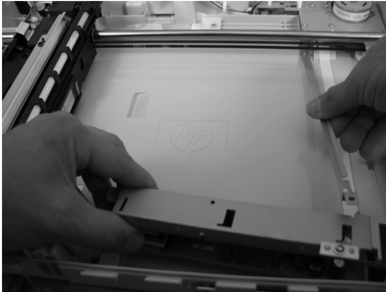
Figure 2-133 Remove the S-ASSY-INV (inverter) (2 of 2)
