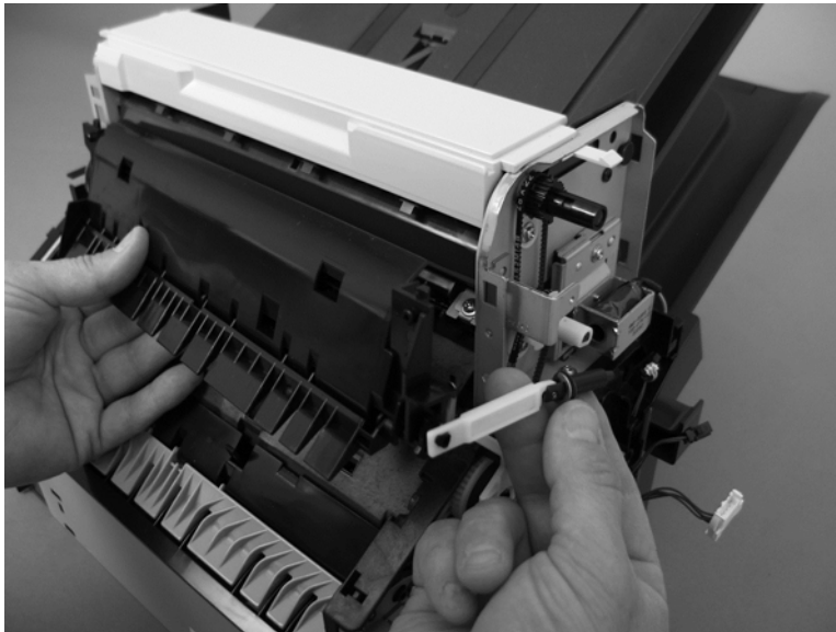
Figure 2-362 Remove the flapper guide assembly (2 of 2)
