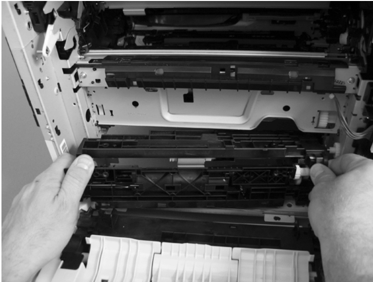
Figure 2-255 Remove the tray-pickup assembly (11 of 11)
