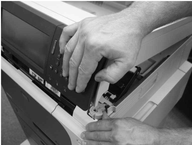
Figure 2-109 Remove the scanner assembly (1 of 6)
