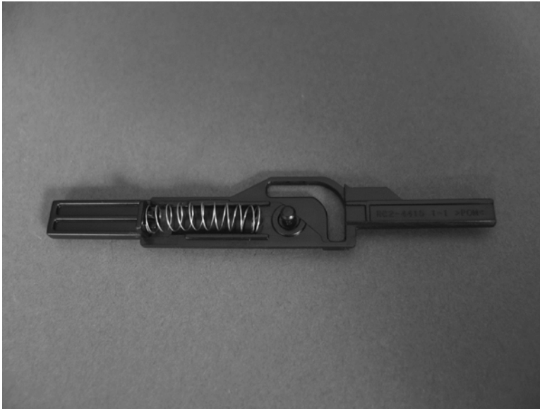
Figure 2-267 Reinstall the PGC actuators (2 of 5)
