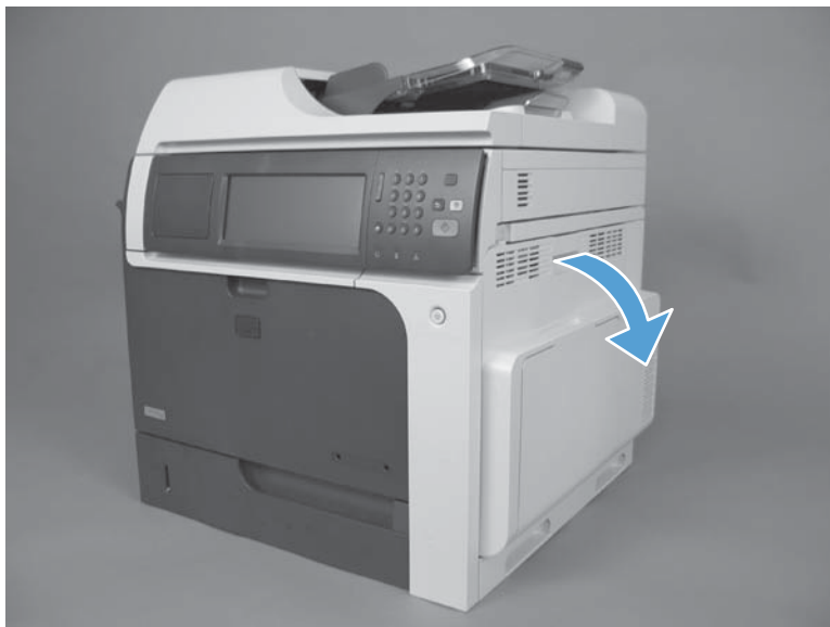
Figure 2-74 Remove the right-door assembly (1 of 9)
