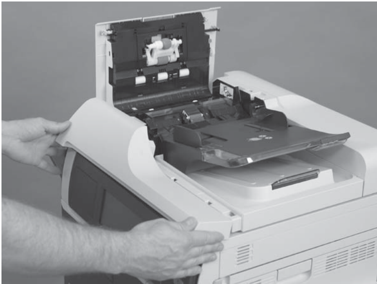
Figure 2-53 Remove ASY-CVR-F-SP (document feeder front cover) (4 of 4)
