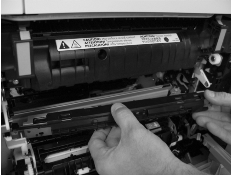
Figure 2-170 Remove the RD sensor assembly (7 of 7)
