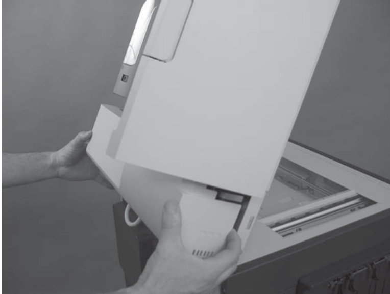
Figure 2-58 Remove the ASY-CVR-F-R-SP (document feeder rear cover) (5 of 5)
