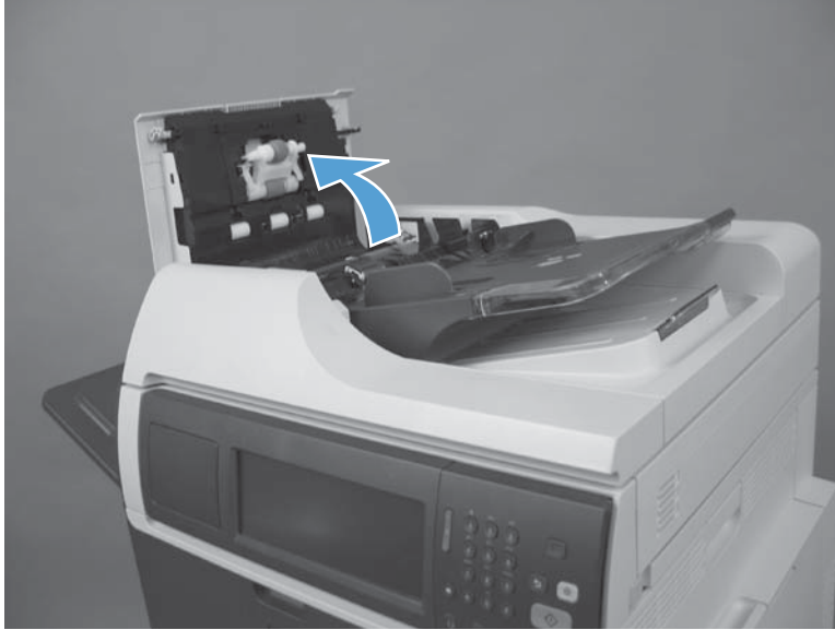
Figure 2-54 Remove the ASY-CVR-F-R-SP (document feeder rear cover) (1 of 5)
