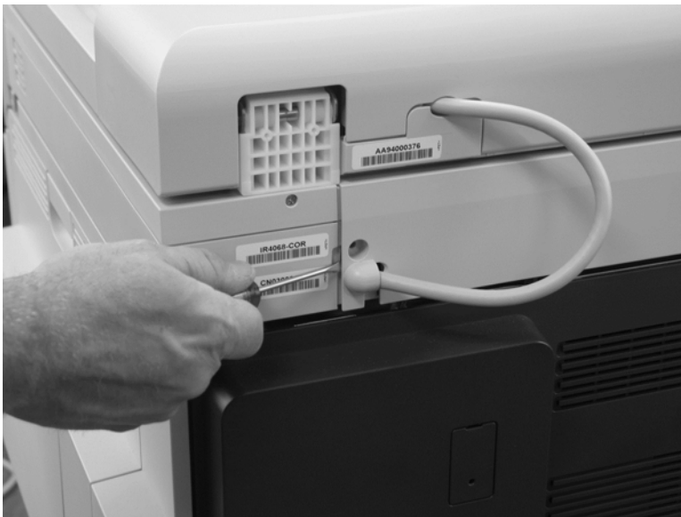
Figure 2-49 Remove S-CVR-REAR (scanner rear cover) (2 of 2)
