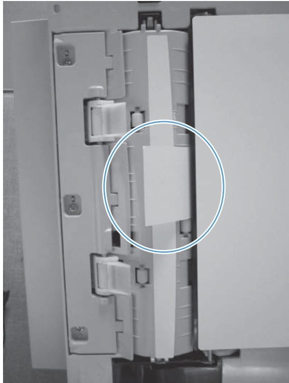
Figure 3-96 Clear the exit sensor with a business card
