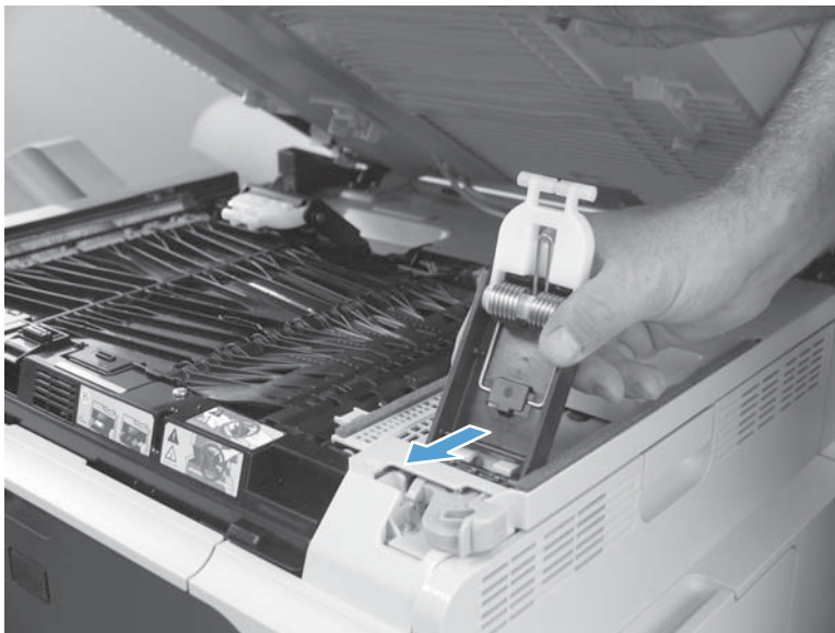
Figure 2-117 Remove the scissor hinge assembly (3 of 3)
