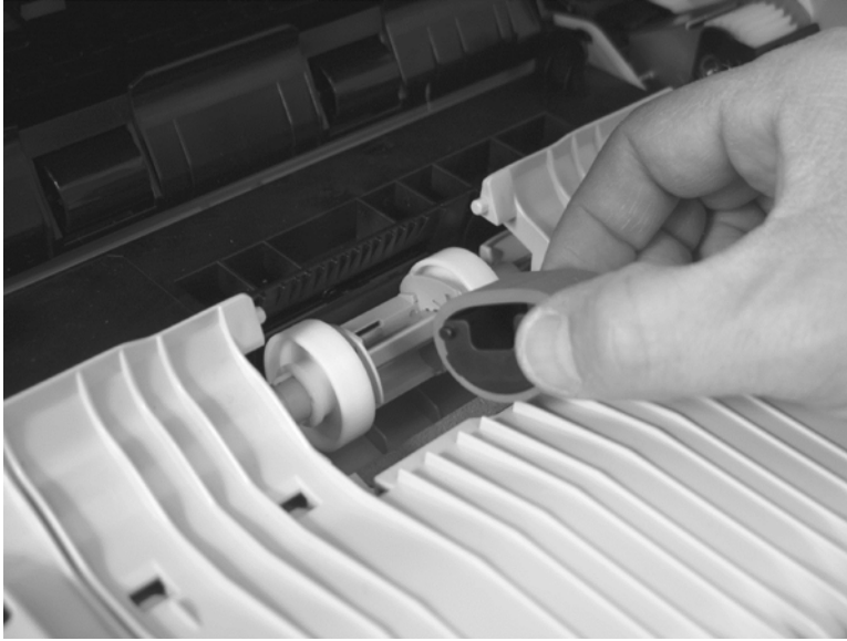
Figure 2-29 Remove the pickup roller (Tray 1) (5 of 5)
