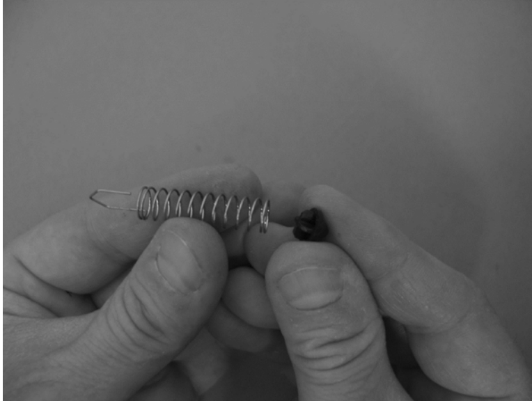
Figure 2-330 Reinstall the lifter assembly (500-sheet paper feeder)
