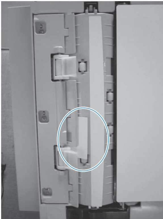
Figure 3-95 Clear the read sensor with a business card
