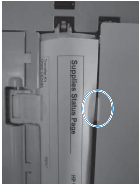
Figure 3-94 Mylar tab causing jam
