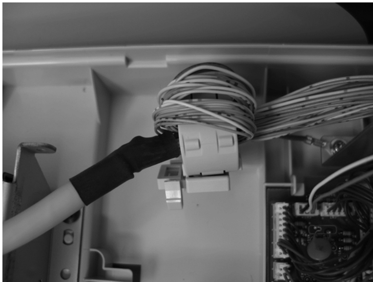
Figure 2-98 Remove the ASM-IF-SP (document feeder cable) (2 of 2)
