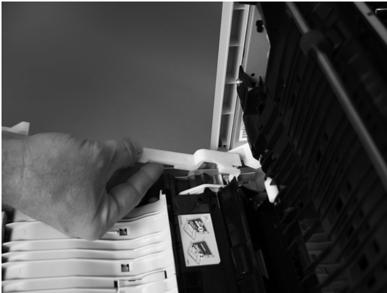
Figure 2-77 Remove the right-door assembly (4 of 9)
