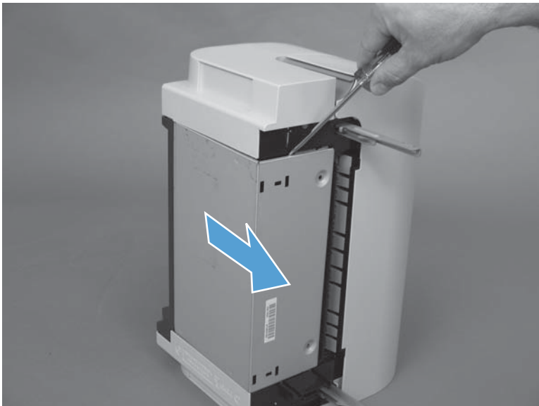
Figure 2-344 Remove the stapling mailbox PCA (2 of 5)
