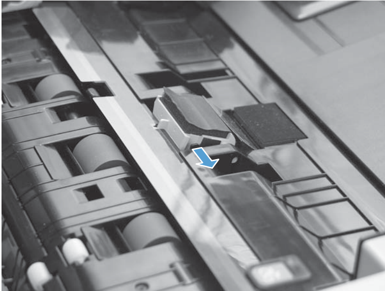
Figure 2-45 Remove the ASY-CVR-FE-PICK-SP (pickup roller cover)
