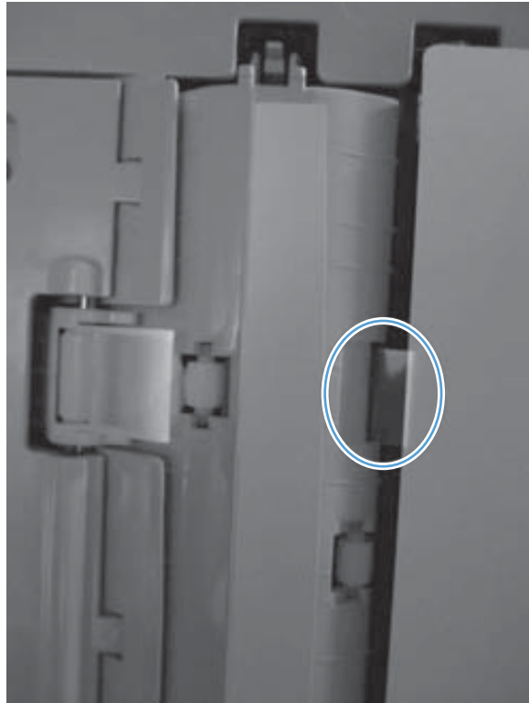
Figure 3-94 Mylar tab causing jam
