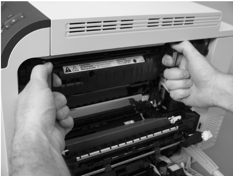
Figure 2-23 Remove the fuser (2 of 2)
