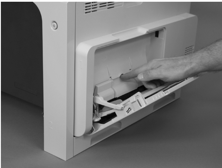
Figure 2-26 Remove the pickup roller (Tray 1) (2 of 5)
