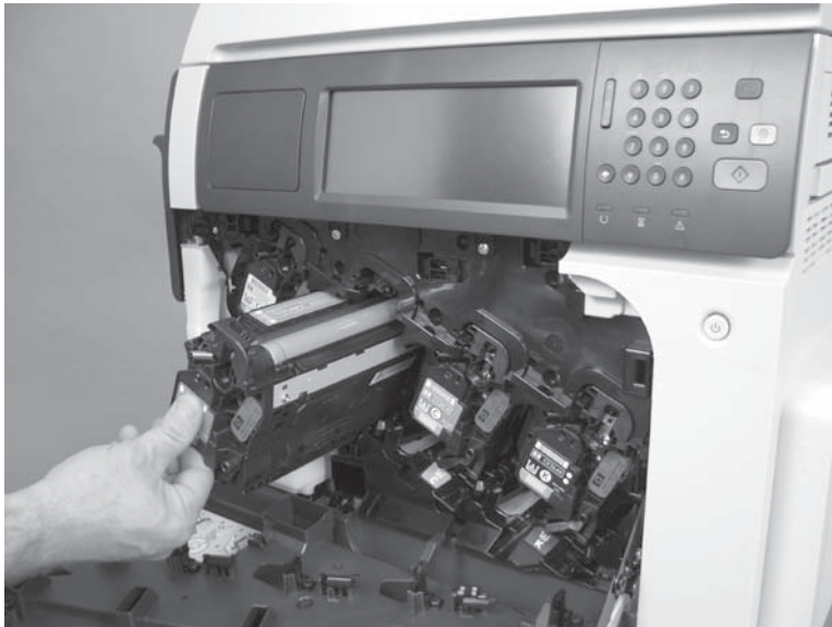
Figure 2-10 Remove the print cartridge (2 of 2)
