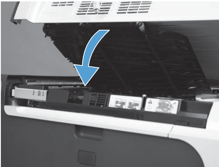
Figure 2-115 Remove the scissor hinge assembly (1 of 3)
