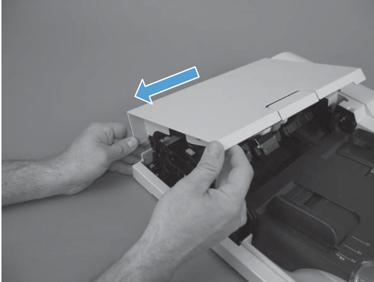
Figure 2-90 Remove the ASY-CVR-FE-FEED-SP (document feeder jam-access cover) (2 of 2)
