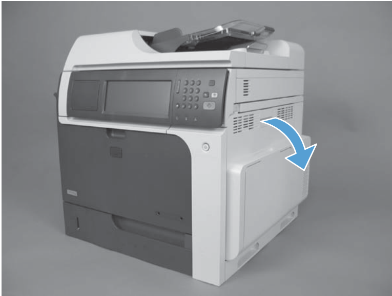
Figure 2-32 Remove the transfer roller (1 of 3)
