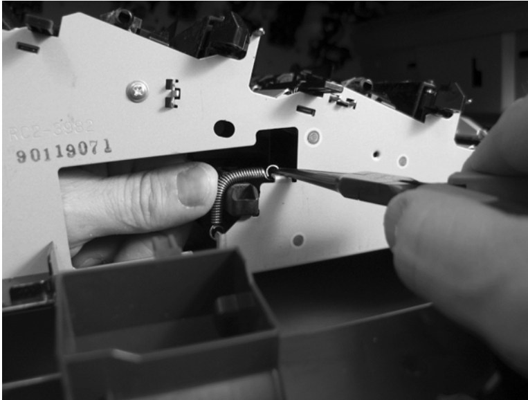
Figure 2-264 Remove the laser/scanner assembly (C/Bk) (4 of 5)
