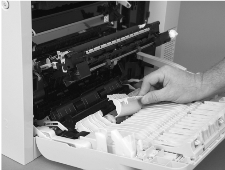
Figure 2-27 Remove the pickup roller (Tray 1) (3 of 5)
