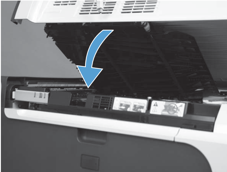
Figure 2-110 Remove the scanner assembly (2 of 6)
