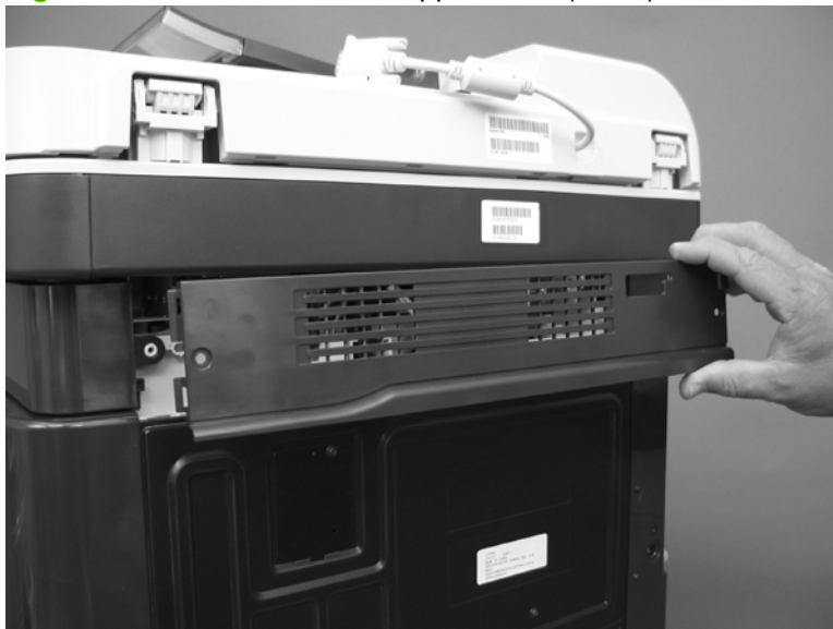
Figure 6-88 Remove the rear-upper cover (4 of 4)
