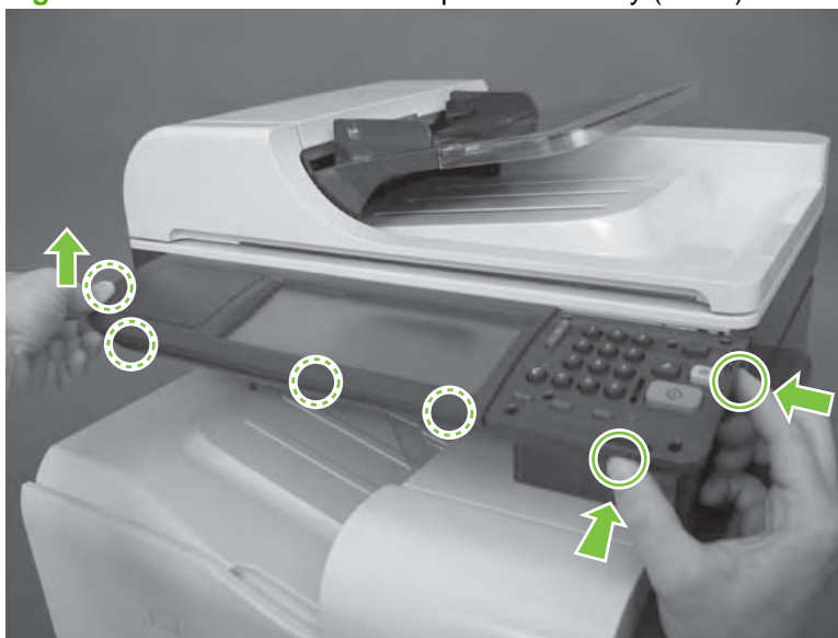
Figure 6-58 Remove the control-panel assembly (1 of 3)
