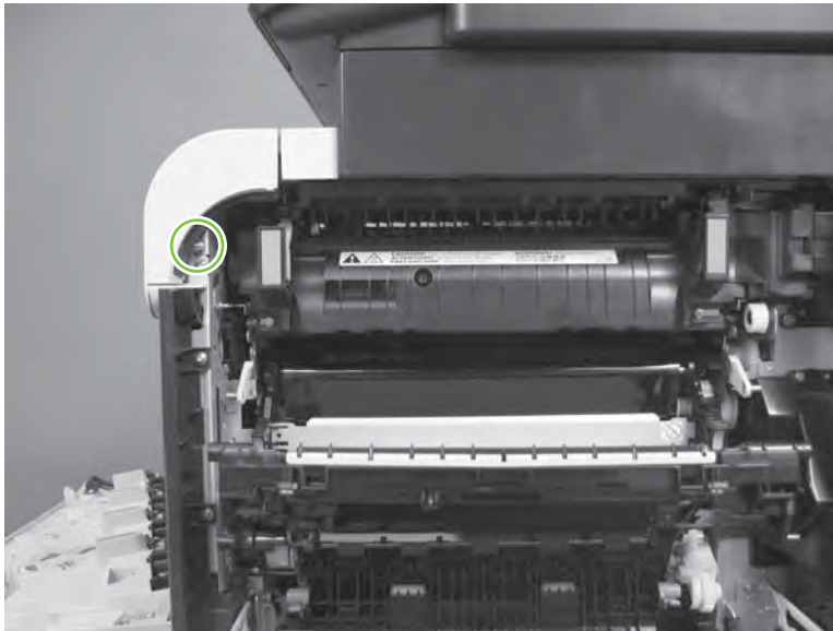
Figure 6-66 Remove the front-upper cover (2 of 4)
