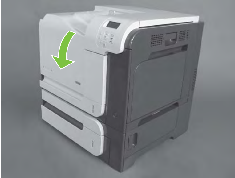
Figure 6-10 Remove the toner-collection unit (1 of 4)
