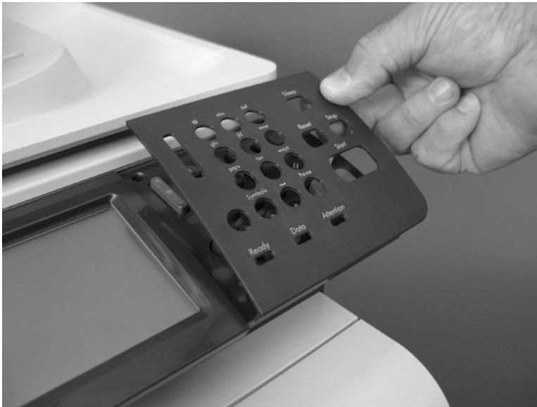
Figure 6-57 Remove the control-panel overlay (2 of 2)
