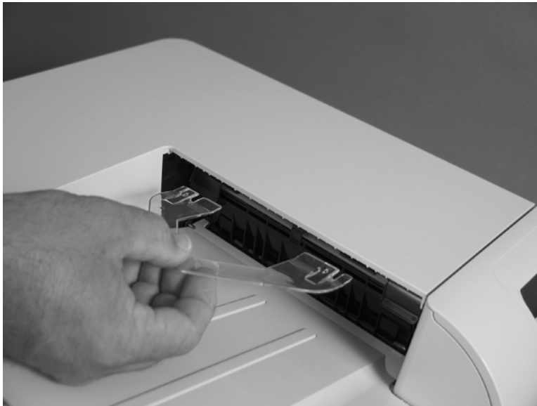
Figure 6-9 Remove the duplex-reverse guide (2 of 2)
