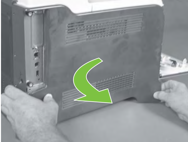
Figure 6-84 Remove the left cover (5 of 5)
