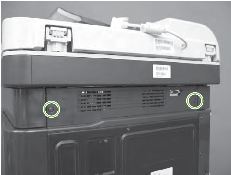
Figure 6-86 Remove the rear-upper cover (2 of 4)
