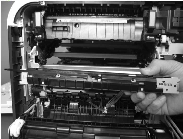
Figure 6-192 Remove the RD sensor assembly (6 of 6)
