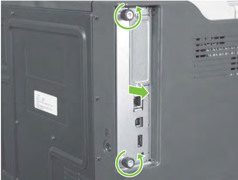
Figure 6-14 Remove the formatter
