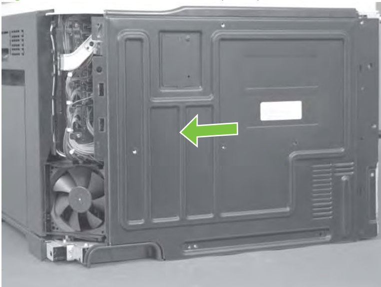
Figure 6-90 Remove the rear cover (2 of 2)
