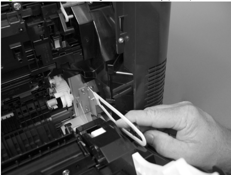
Figure 6-72 Remove the right-door assembly (4 of 8)
