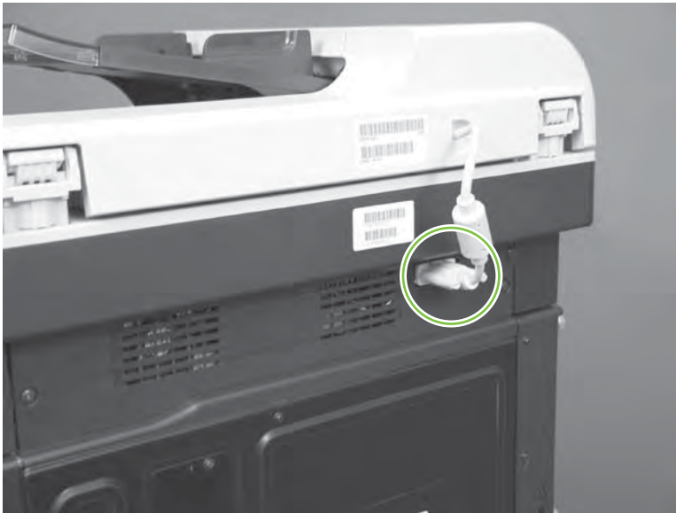
Figure 6-85 Remove the rear-upper cover (1 of 4)
