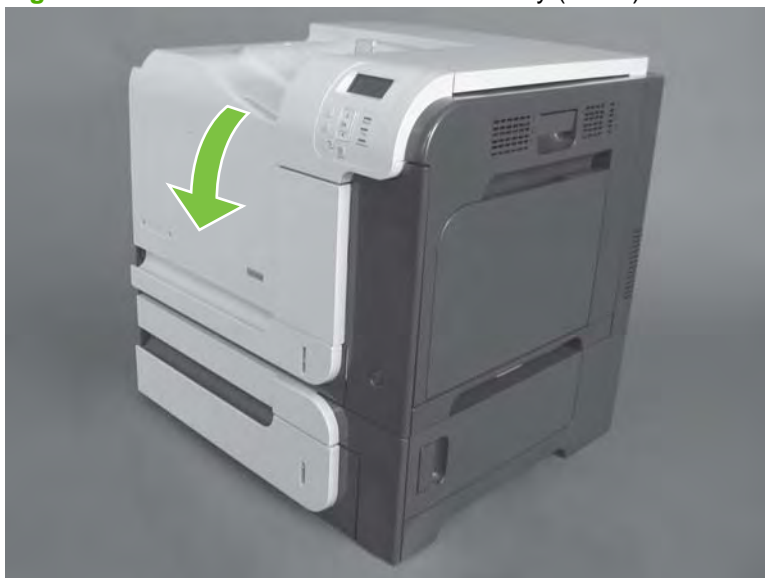
Figure 6-44 Remove the front-door assembly (1 of 2)
