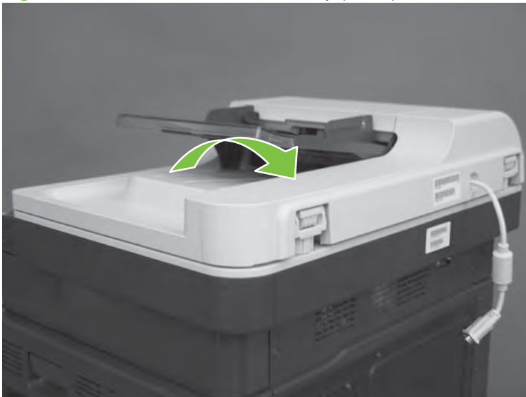
Figure 6-47 Remove the ADF assembly (2 of 4)
