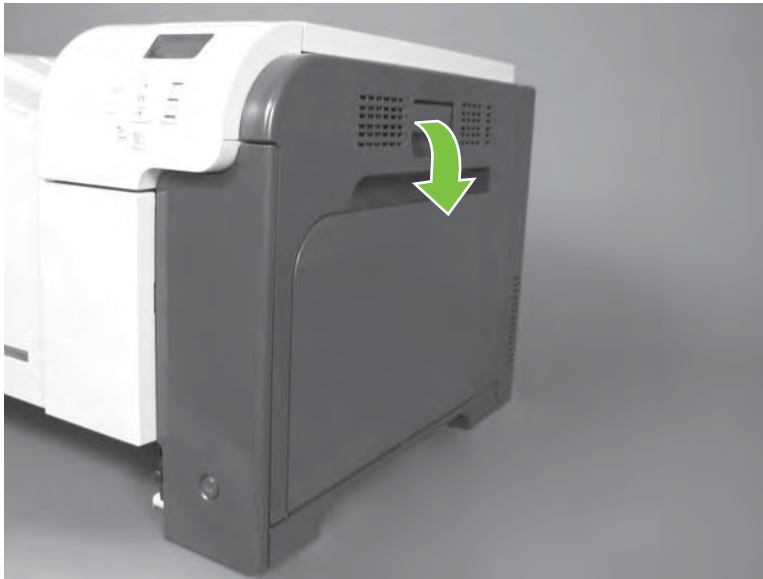
Figure 6-69 Remove the right-door assembly (1 of 8)
