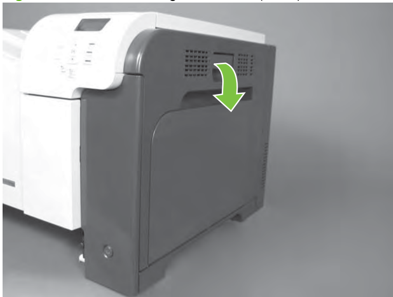
Figure 6-77 Remove the right-rear cover (1 of 3)
