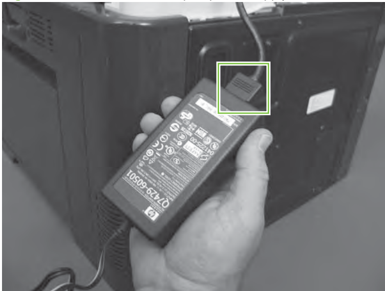
Figure 6-136 Remove the stapler power supply
