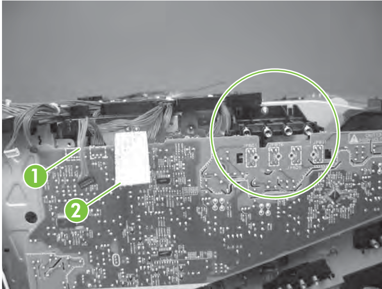
Figure 6-260 Reinstall the high-voltage power supply upper
