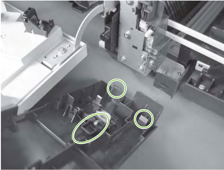
Figure 6-93 Remove the right-front cover (3 of 5)
