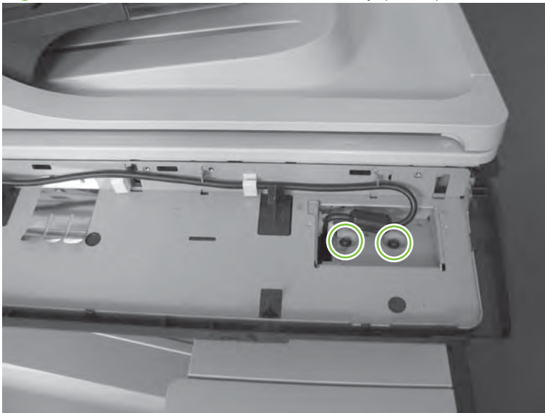
Figure 6-97 Remove the scanner assembly (1 of 6)
