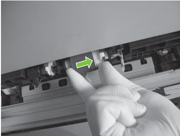
Figure 6-27 Remove the pickup roller (Tray 2) (2 of 4)
