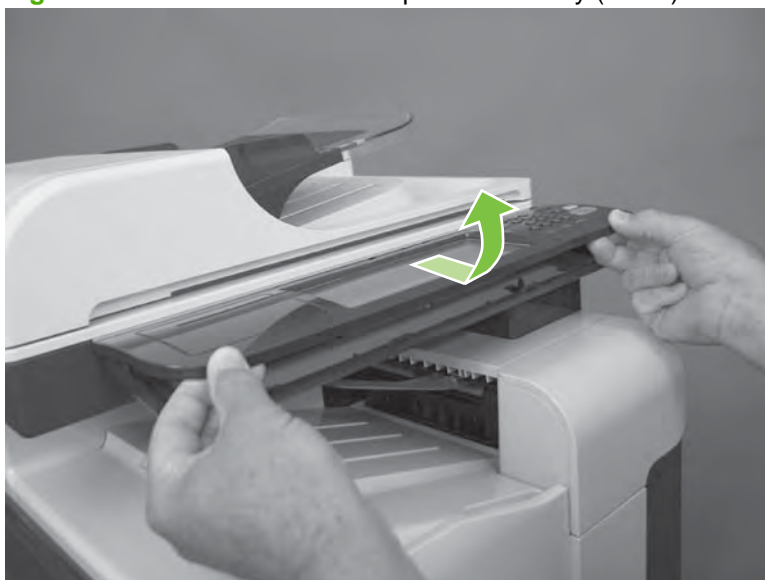
Figure 6-59 Remove the control-panel assembly (2 of 3)
