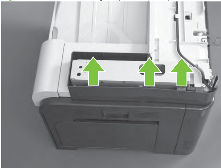
Figure 6-126 Remove the right-top cover (3 of 5)
