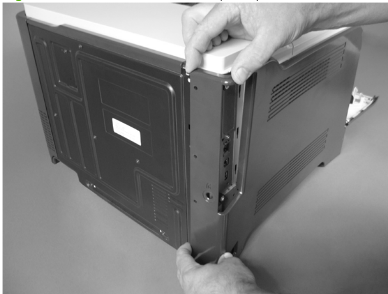
Figure 6-81 Remove the left cover (2 of 5)
