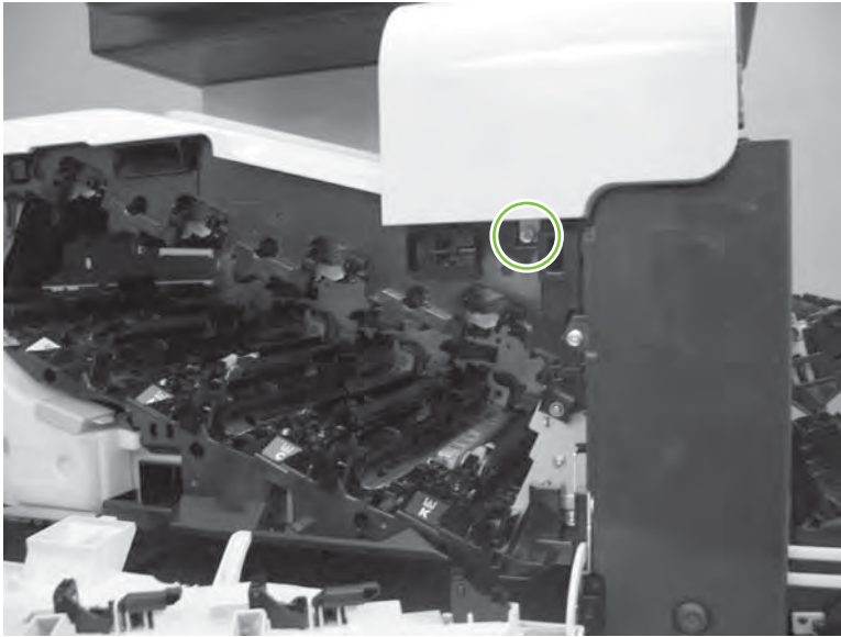
Figure 6-67 Remove the front-upper cover (3 of 4)
