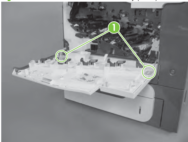
Figure 6-45 Remove the front-door assembly (2 of 2)
