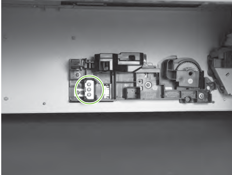
Figure 7-26 Test the optional Tray 3 media-size sensors
