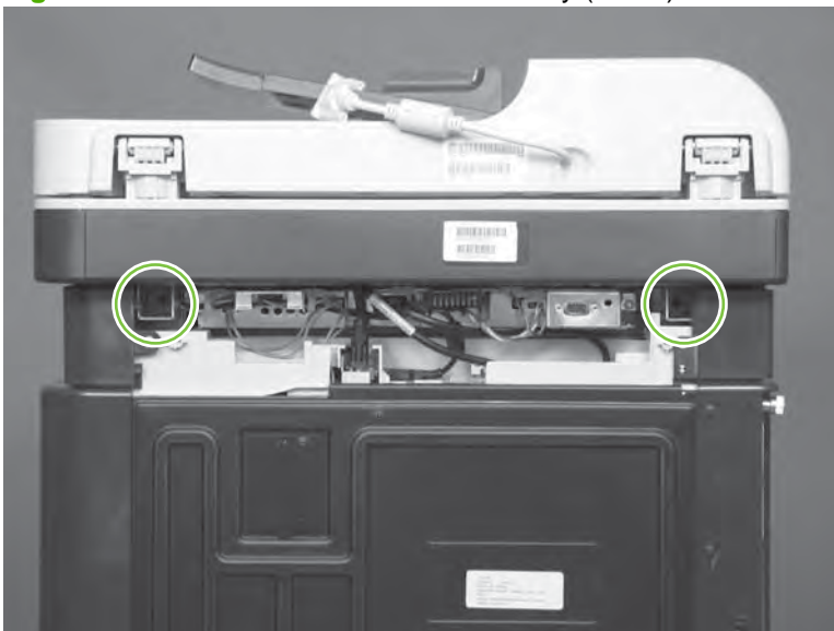
Figure 6-98 Remove the scanner assembly (2 of 6)
