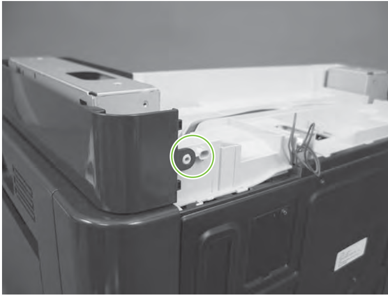
Figure 6-125 Remove the right-top cover (2 of 5)
