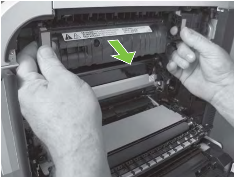
Figure 6-25 Remove the fuser (2 of 2)
