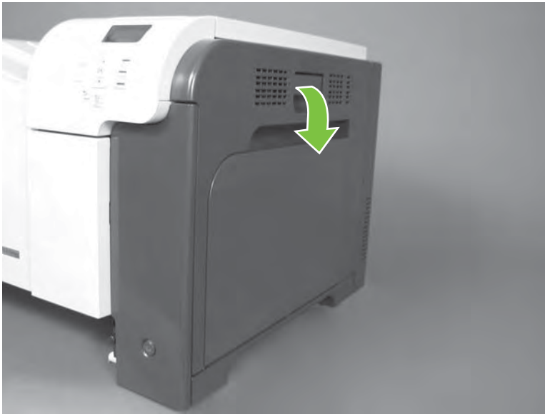
Figure 6-24 Remove the fuser (1 of 2)
