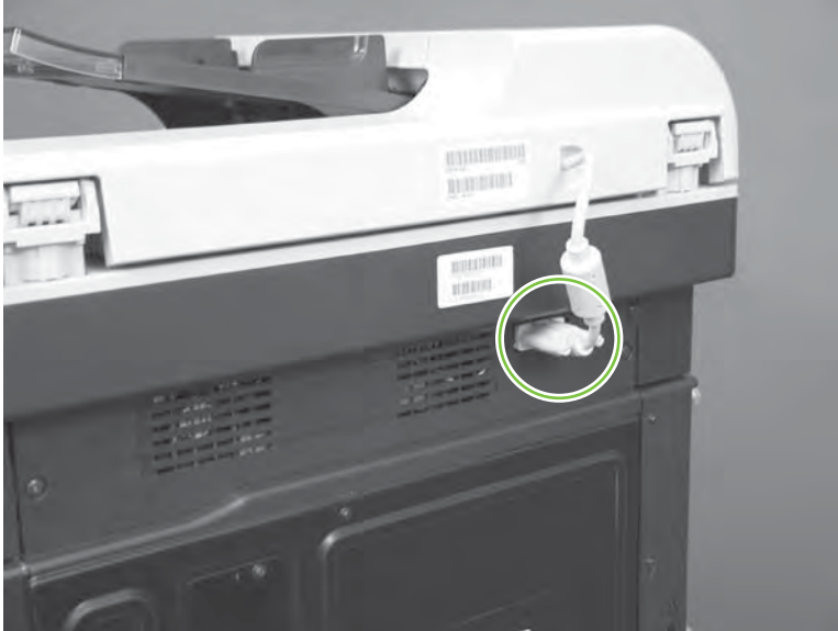
Figure 6-46 Remove the ADF assembly (1 of 4)
