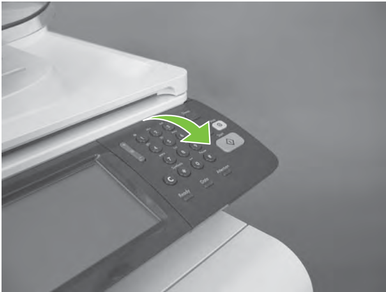
Figure 6-56 Remove the control-panel overlay (1 of 2)
