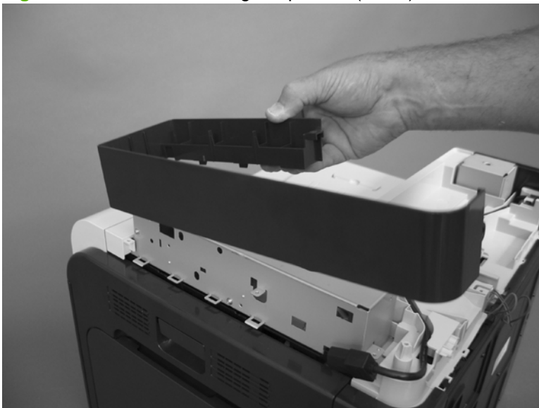
Figure 6-128 Remove the right-top cover (5 of 5)
