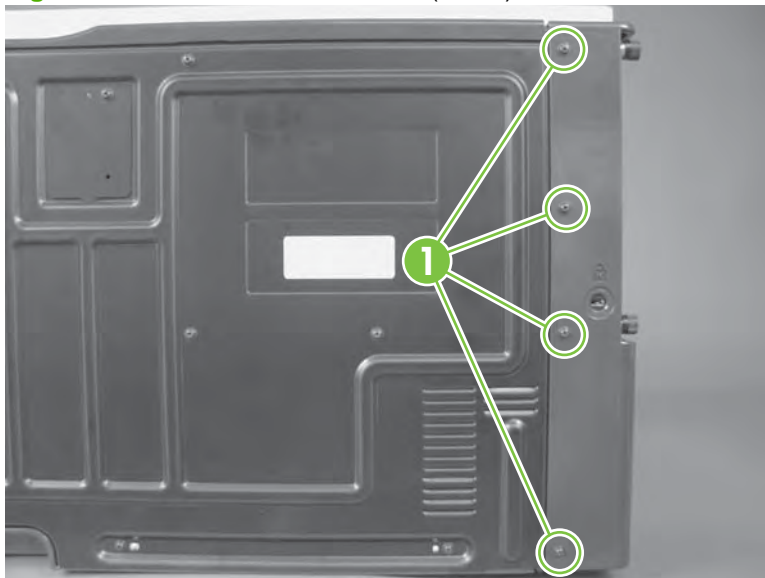
Figure 6-80 Remove the left cover (1 of 5)
