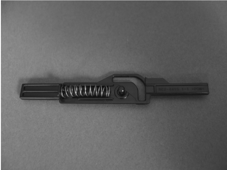
Figure 6-251 Reinstall the PGC actuators (2 of 5)
