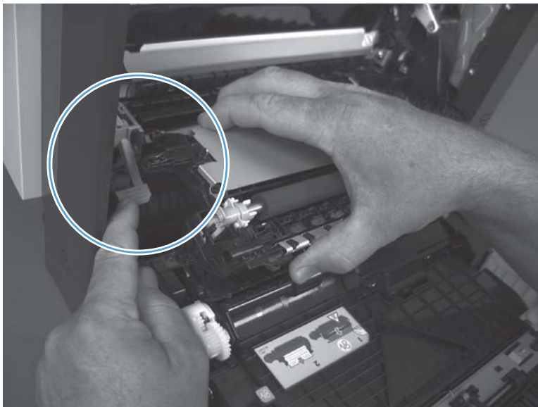
Figure 1-155 Reinstall the secondary transfer assembly
