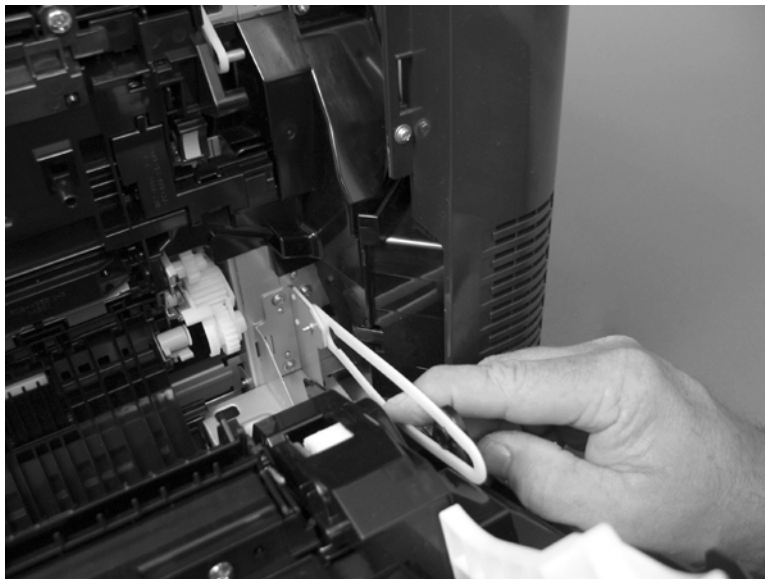
Figure 1-61 Remove the right-door assembly (4 of 8)
