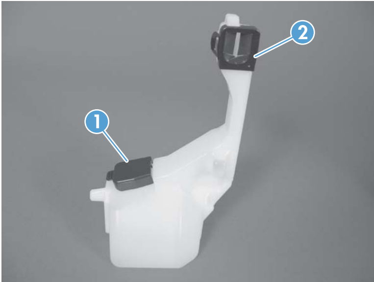
Figure 2-11 Remove the toner collection unit (4 of 4)
