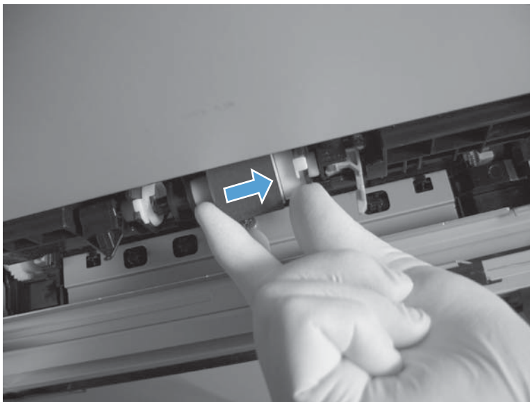
Figure 2-24 Remove the pickup roller (Tray 2; 2 of 4)
