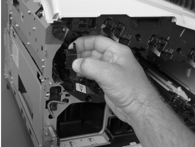
Figure 2-100 Remove the residual toner feed motor (2 of 7)
