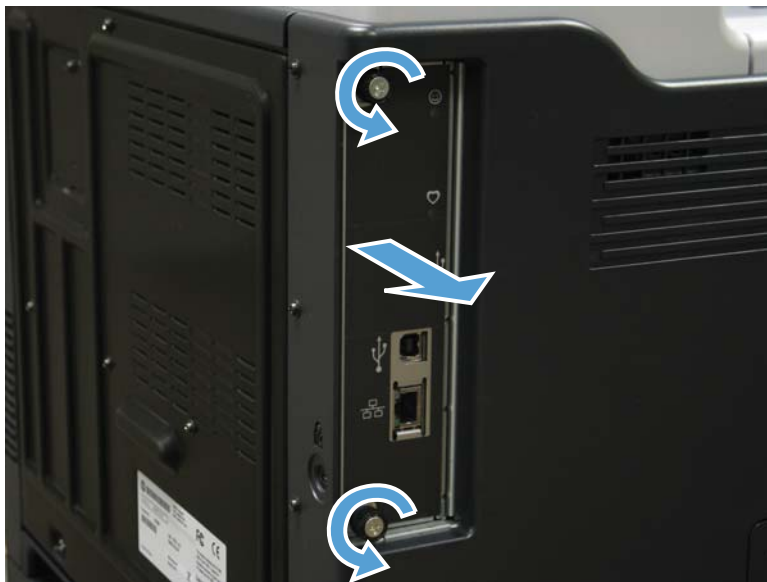
Figure 2-12 Remove the formatter
