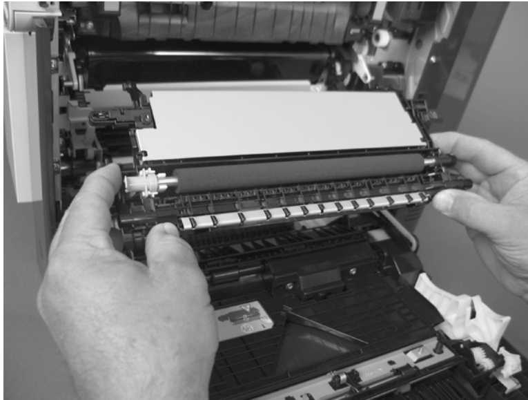
Figure 2-36 Remove the secondary transfer assembly (3 of 3)
