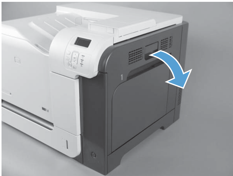
Figure 2-55 Remove the right rear cover (1 of 3)
