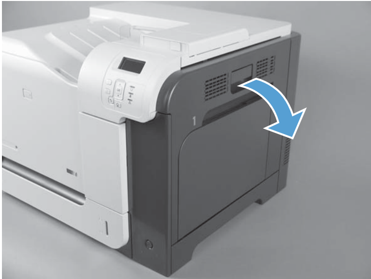
Figure 2-47 Remove the right door assembly (1 of 8)
