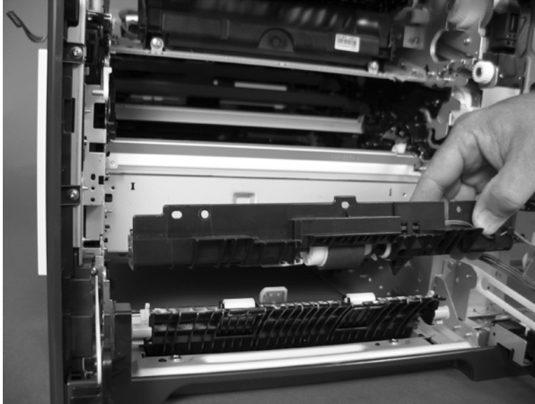
Figure 2-165 Remove the cassette pickup assembly (3 of 3)
