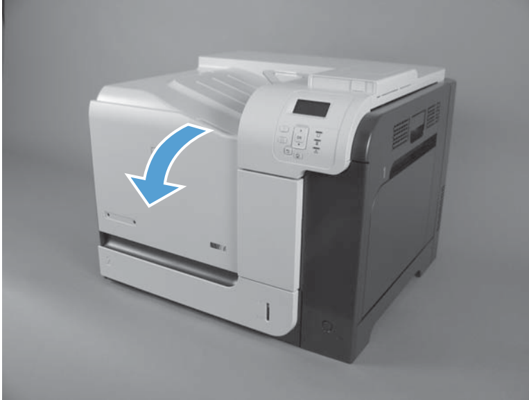
Figure 2-4 Remove the print cartridge (1 of 2)
