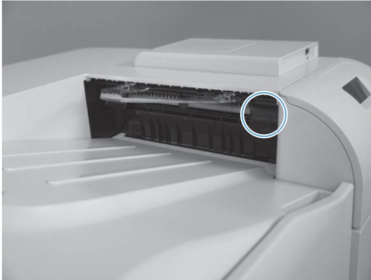
Figure 3-10 Test the output-bin-full sensor
