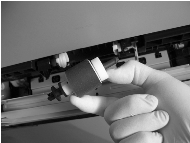
Figure 2-26 Remove the pickup roller (Tray 2; 4 of 4)
