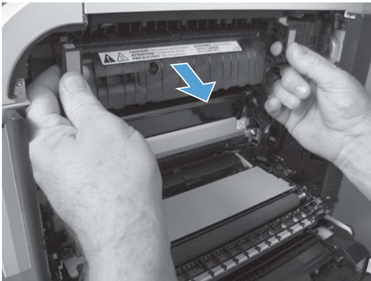
Figure 2-20 Remove the fuser (2 of 2)
