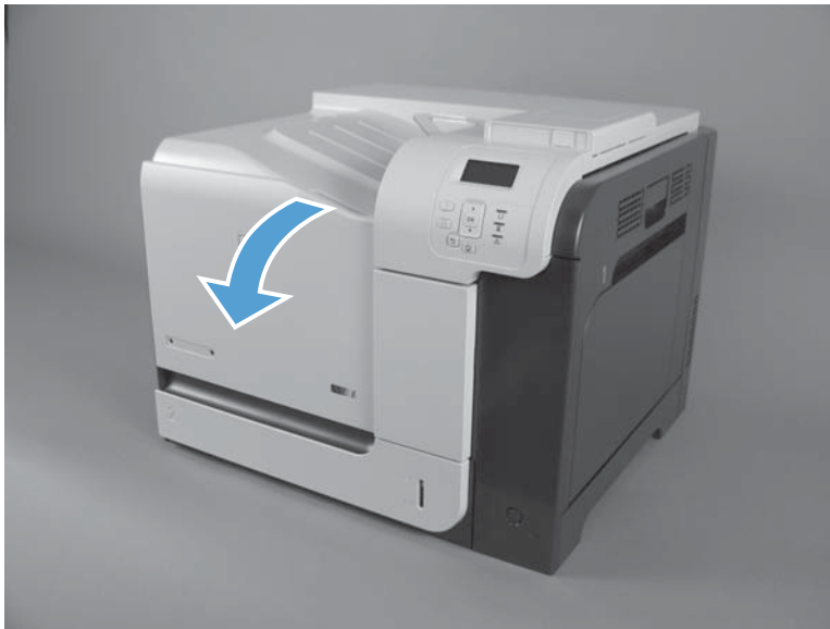
Figure 2-45 Remove the front door assembly (1 of 2)
