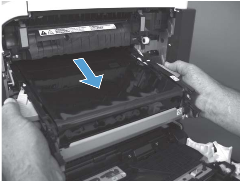
Figure 2-40 Remove the intermediate transfer belt (3 of 3)
