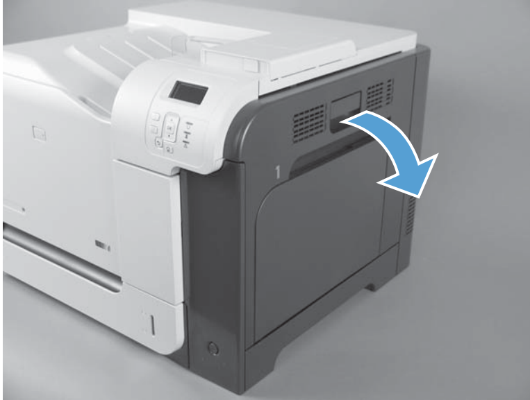
Figure 2-19 Remove the fuser (1 of 2)
