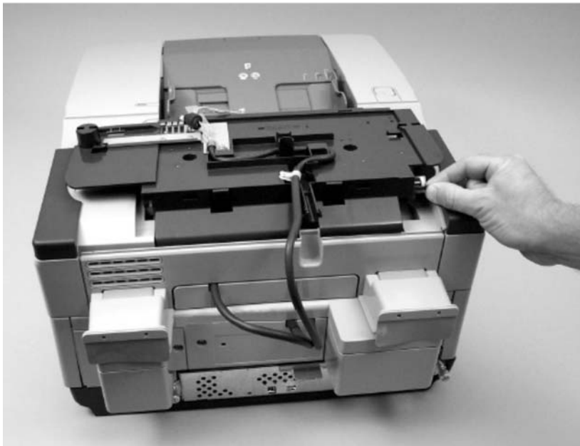
Figure 5-35 Removing the control-panel cover assembly (4 of 6)
