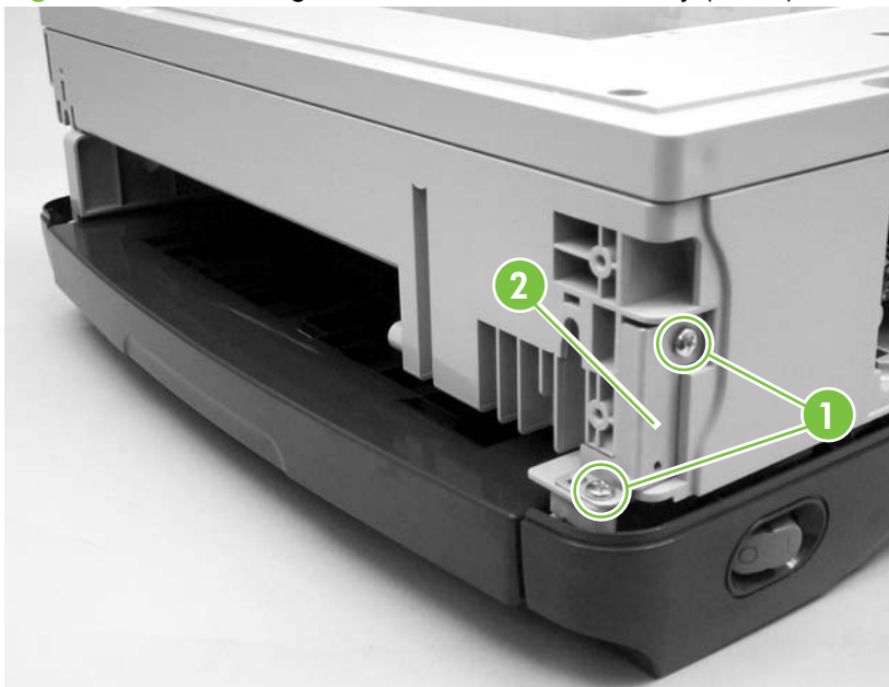
Figure 5-78 Removing the flatbed scanner assembly (1 of 4)
