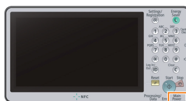
Pattern 1 (The Main Power LED blinks 2 times in 4 seconds: Controller error)
