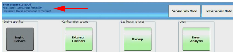
[15] 11506 in Service screen and engine off
