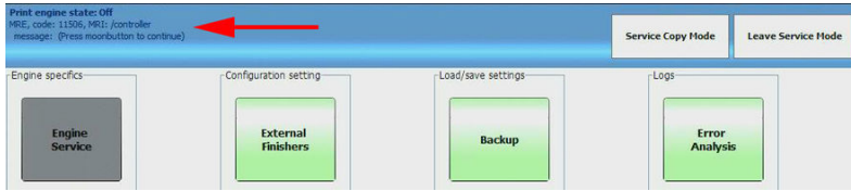
Fig. 11506 in Service screen and engine off
