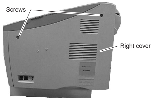
Figure 5-24 Preparation for Installation 1
