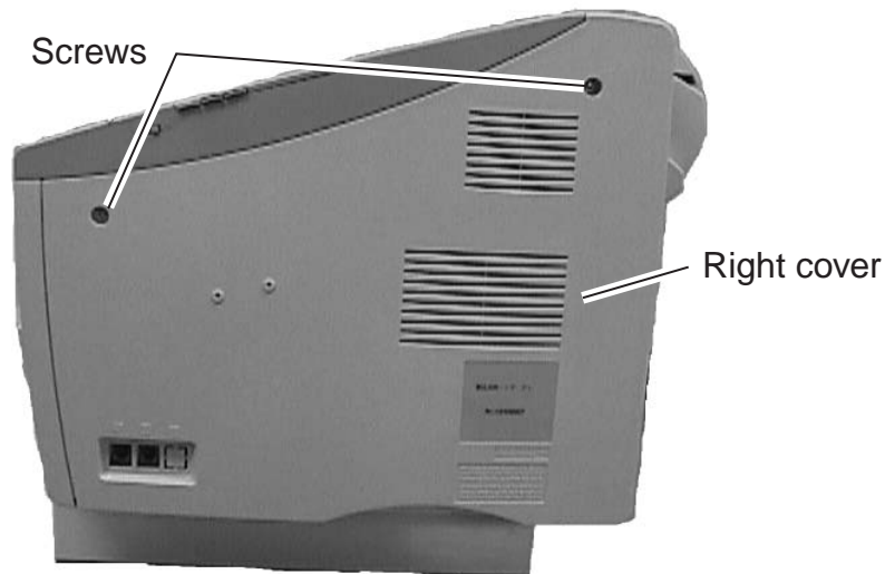
Figure 5-73 Preparation for Installation 1
