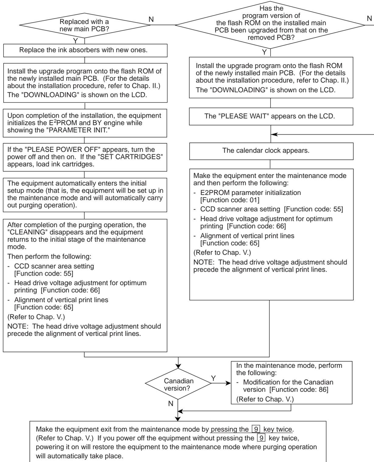
When replacing the main PCB, it is recommended to replace all ink cartridges in order to maintain accurate ink level information.
