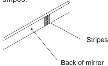
The non-marked sides of the mirrors A and C should face towards the rear of the scanner frame ASSY; the non-marked side of the mirror B should face to the front.
