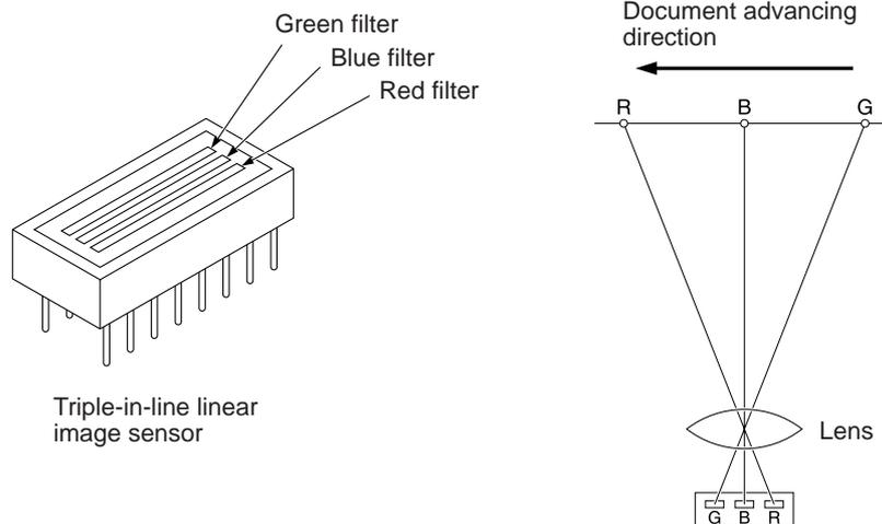
The number of scan lines between the green and blue scanning start positions and between the blue and red scanning start positions is eight. The scanner retains 16 scan lines of green image and eight scan lines of blue image. The moment a red image is captured, the scanner superimposes all of those three color data of a same scan line to generate a full-color image.
