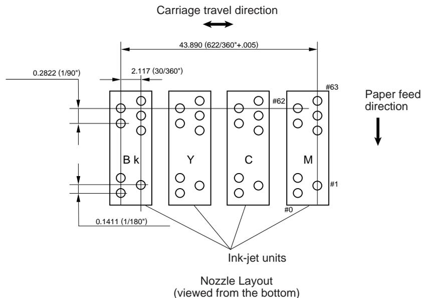
As the carriage holding the print head travels at the printing speed, the character generator sends print command pulses to the circuits driving the piezoelectric actuators embedded in the print head.
