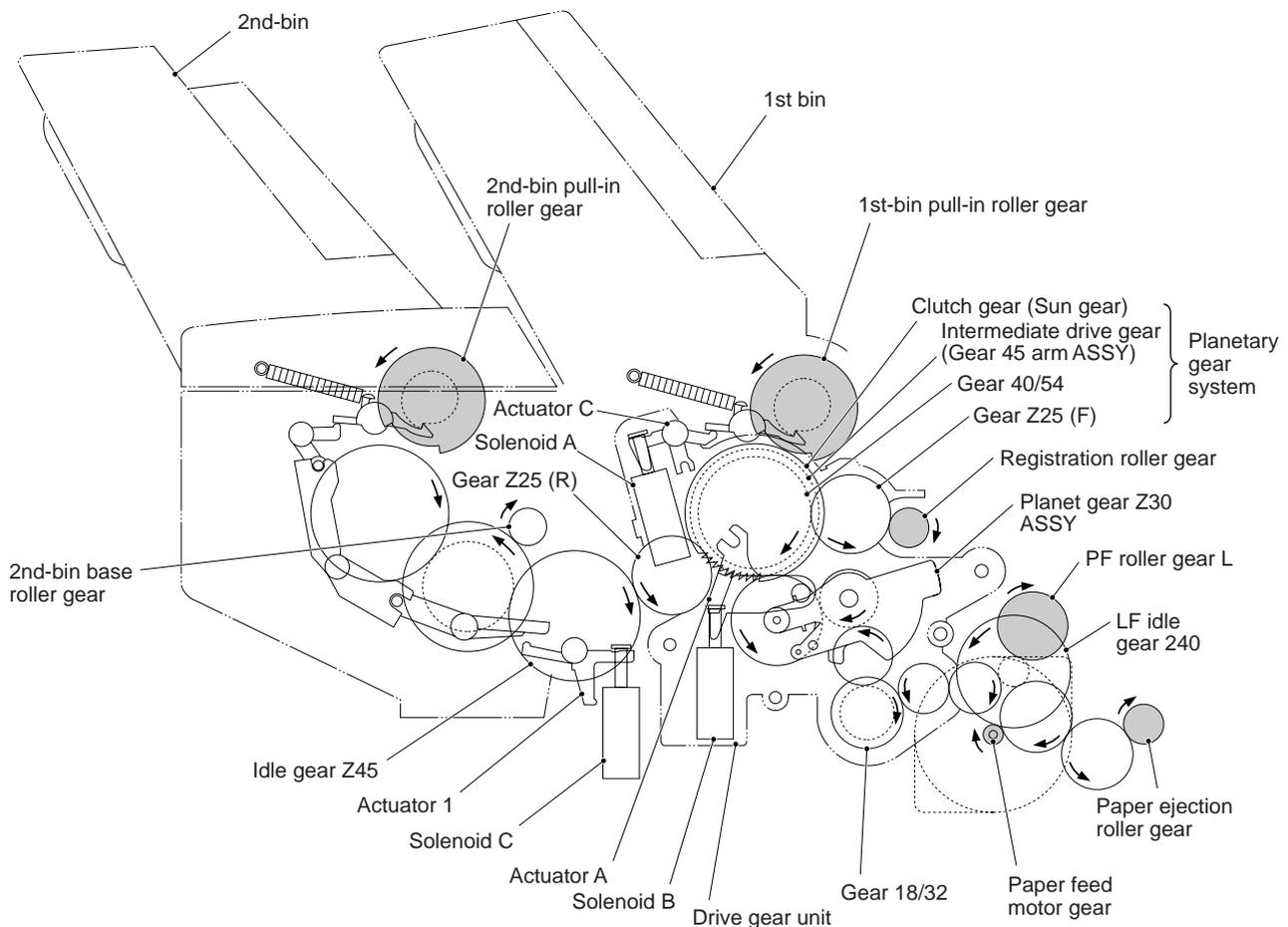
The paper pulling-in and registration mechanism consists of the 1st bin, 1st-bin pull-in roller ASSY, 2nd bin, 2nd-bin pull-in roller ASSY, 2nd-bin base roller ASSY, registration roller ASSY, LF chute ASSY, paper pressure chute ASSY, paper feed roller, paper ejection roller ASSY, and sensors.
