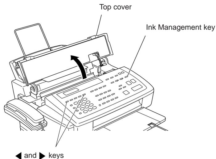
The carriage automatically moves left to the ink cartridge replacement position.
