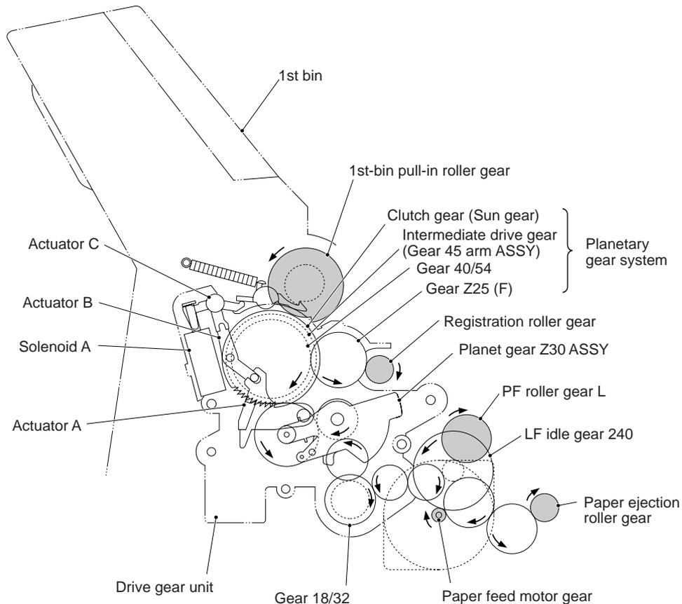
The paper pulling-in and registration mechanism consists of the 1st bin, 1st-bin pull-in roller ASSY, registration roller ASSY, LF chute ASSY, paper pressure chute ASSY, paper feed roller, paper ejection roller ASSY, and sensors.
