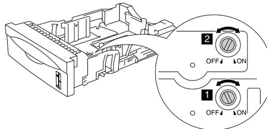
The switches in this illustration are shown in the default setting position.
