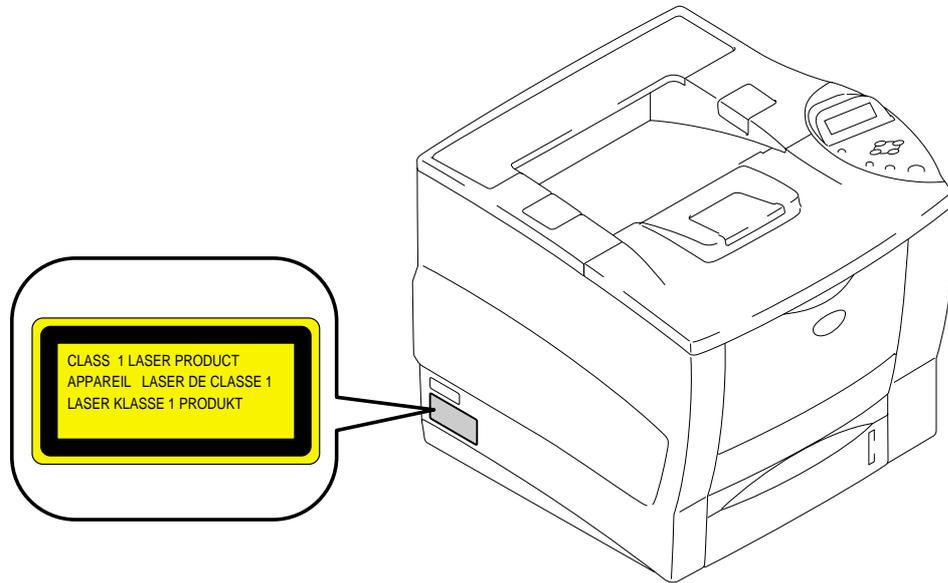
This printer has a laser diode which emits invisible laser radiation in the Laser Unit. The Laser Unit should not be opened without disconnecting the two connectors connected with the AC power supply and laser unit. Since the variable resistor in the laser unit is adjusted in accordance with the standards, never touch it.
