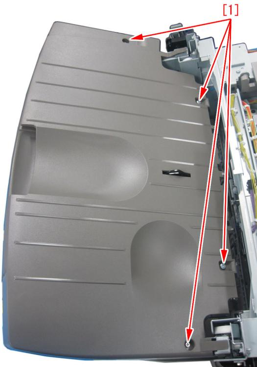
1-9) Remove 5 screws [1] on the undersurface of the Tray 1.
