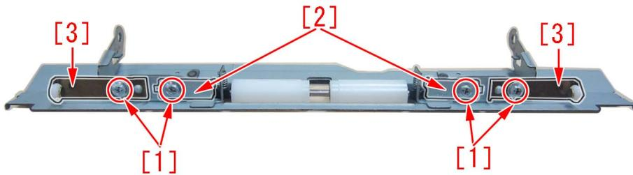
4) Remove the roller [1], 2 bushings [2] and 2 compression springs [3] from the deck pull-out roller feed guide.
