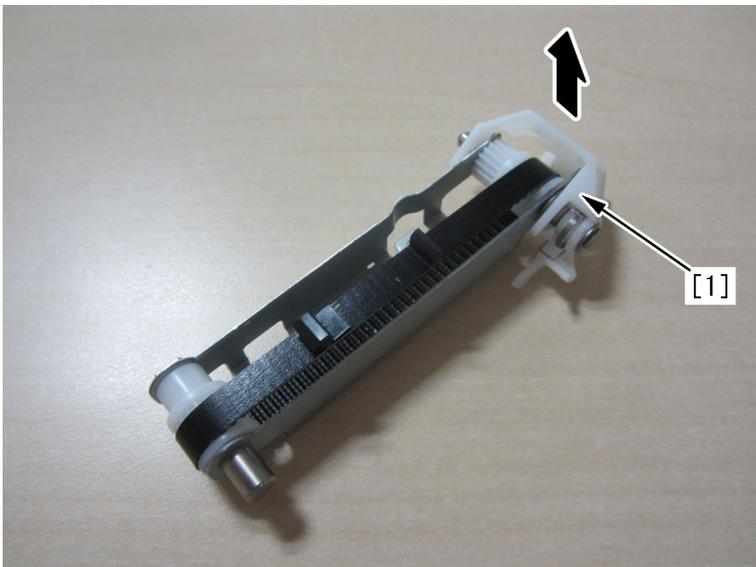
13) Remove the clip [1] and the E-ring [2] from the back end assist unit, and replace the timing belt [3] with the new type.
