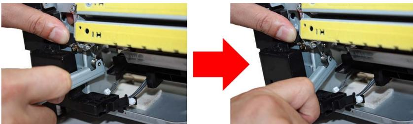
[Note] To attach the spring, put the looped end [a] in the boss [b]. Do not put the looped portion at the center [c] in the boss [b]. The photo [A] indicates the proper way to attach the spring and [B], an erroneous way to attach the spring.
