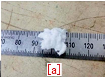
[Reference] Applying grease is not necessary to the area [a], approximately 10mm between the root of the gear. However, there is no problem if the grease is applied to this area.
