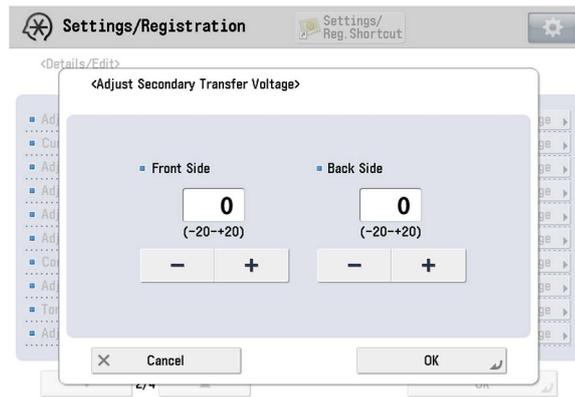
7. Select Front Side in the adjust secondary transfer voltage screen, press "+" button five times and if the corrected value[a] is confirmed to be "+5", then press "OK".
