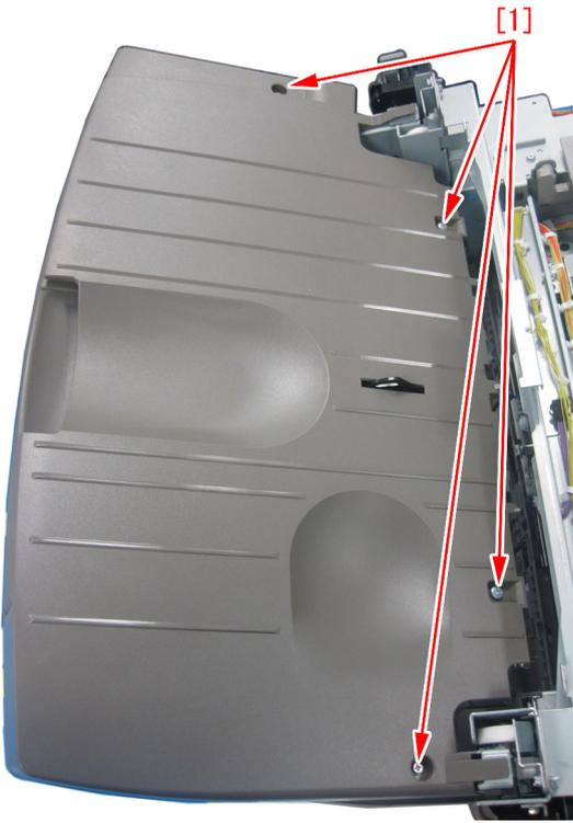
2-12) Remove 5 screws [1] on the underside of the Tray 1.
