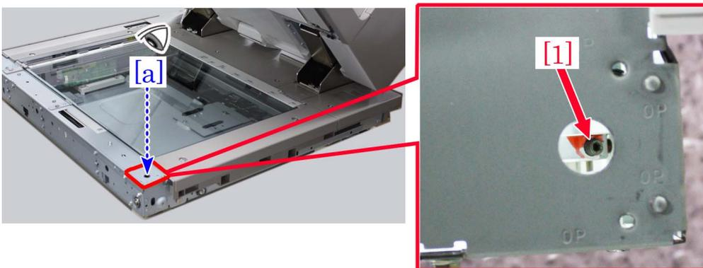
Appearance of a screw [1] of the drive pulley on the front from the right side [b]
