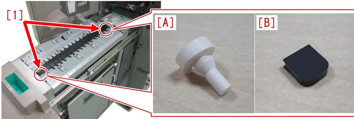
6) Attach the spacers in the arrow side [c] of the reference lines [a] and [b]. A deviation up to +2mm in the arrow side [c] can be tolerated.
