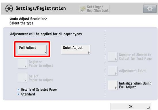
11) Select a paper source of the paper type that needs to undergo the correction, and press "OK". According to the message appearing on the screen, output a test print and scan it, and perform Full Adjust.
