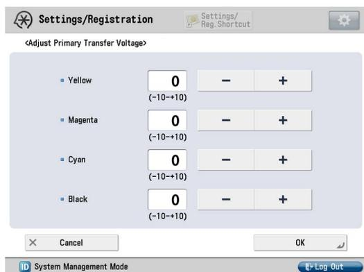
7) Select yellow, magenta and cyan in the adjust primary transfer voltage screen, press "-" button thrice and if the corrected value[a] is confirmed to be "-3", then press "OK".
