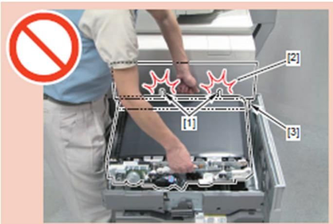
12) Hold 2 handles [1] and align the right edge [A] and the left edge [B] of the ITB unit with the 2 markings [2], and then place the ITB unit [3] horizontally.
