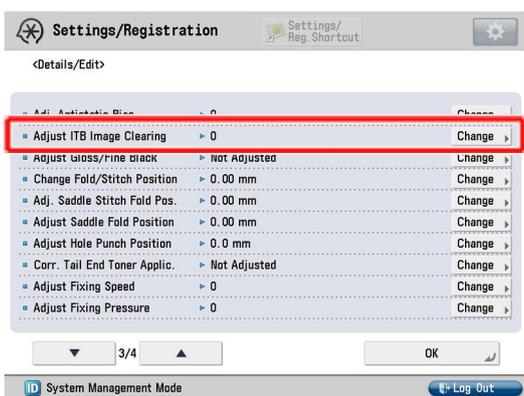
[Points to note] If the control panel does not display Adjust ITB Image Cleaning, change the parameter of Service mode > Mode List > COPIER > Option > DSPLY-SW > IMGC-ADJ to "1" and perform a power cycle of main-power (OFF/ON). The default value is "0".
