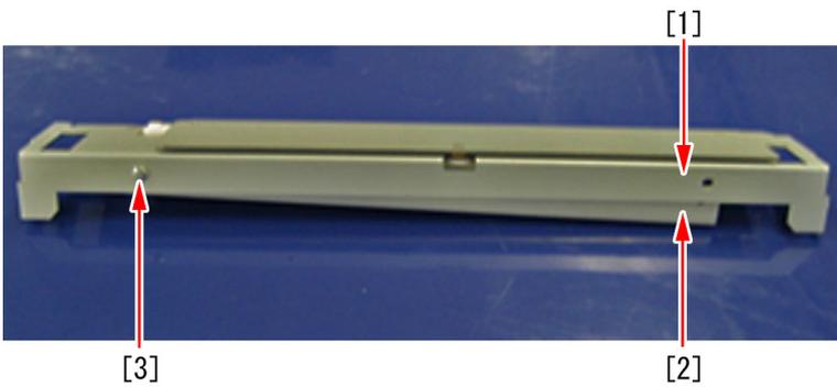
2-33) Remove the 4 screws and remove the metal plate unit.
