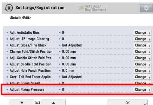
10) Select Adjust Fixing Pressure. Using the "button, change the correction value [a] to "-3" and press "OK".
