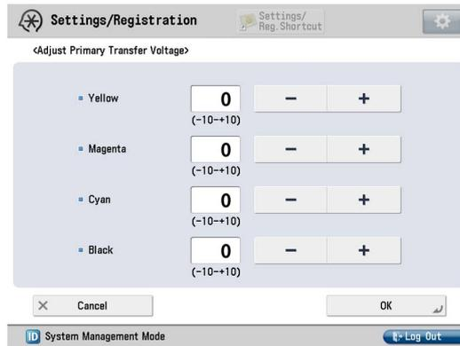
7. Select Cyan and Black in the adjust primary transfer voltage screen, press "-" button thrice and if the corrected value[a] is confirmed to be "-3", then press "OK".
