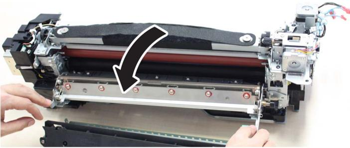
3) Remove the 2 torsion springs [1] and the 1 metal sheet [2].
