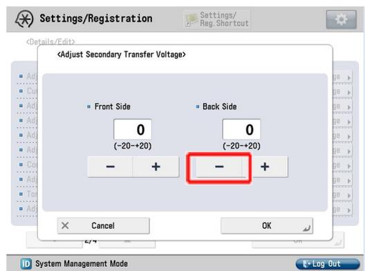
[Caution] Changing this setting reduces the secondary transfer voltage, therefore an image of high density may come out lighter or void may occur on the trailing edge.
