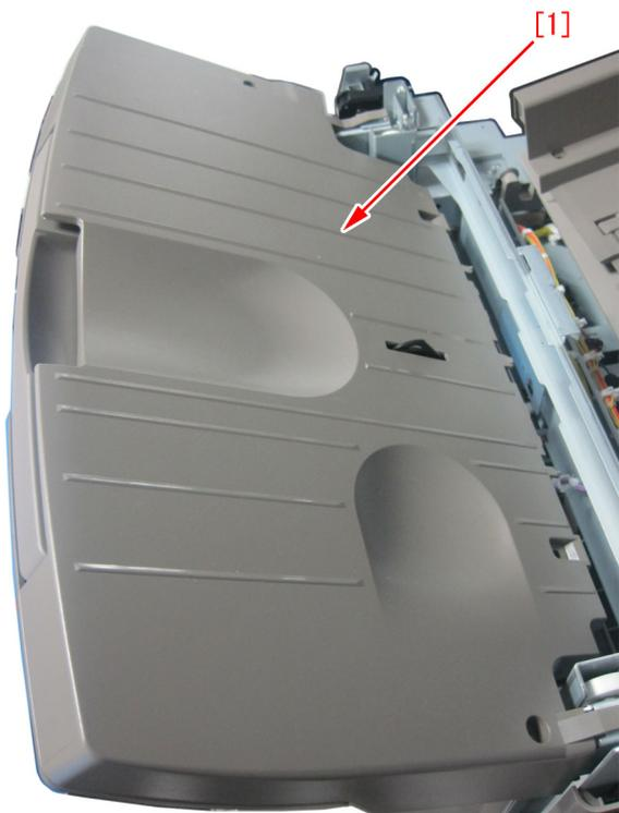
2-14) Check the safety cover to return the come off parts to the original position.
