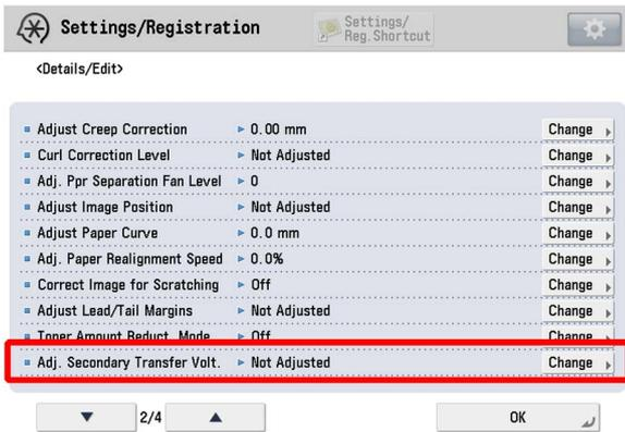
6) If the adjust secondary transfer voltage screen is displayed, the presetting is completed.
