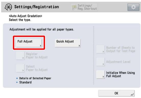
9) Select a paper source of the paper type that needs to undergo the correction, and press "OK". According to the message appearing on the screen, output a test print and scan it, and perform Full Adjust.
