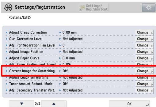
6) In the adjusting screen of correct image for scratching, select "ON" and press "OK".
