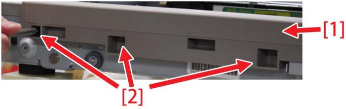
Remove the 4 screws [2] and remove the metal plate A [1].
