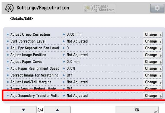
17) Select a paper source of the paper type that needs to undergo the correction, and press "OK". According to the message appearing on the screen, output a test print and scan it, and perform Full Adjust.
