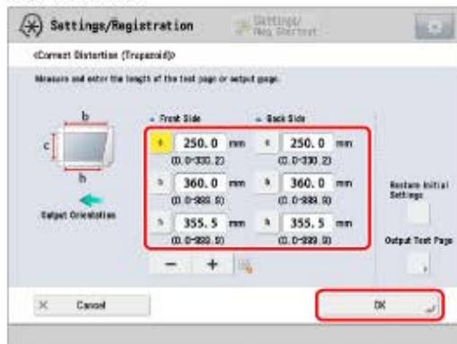
[c]: Enter the measured length from the left side lead edge of the printing area to the right side lead edge of the printing area.
