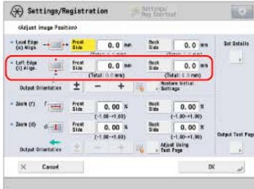
For example, if the measured length of 'l' is 21.0 mm, enter - 1.0 mm for <Left Edge (l) Align.>. For example, if the measured length of 'l' is 19.0 mm, enter + 1.0 mm for <Left Edge (l) Align.>. The 1.0 mm difference between the measured value and the default value is corrected.
