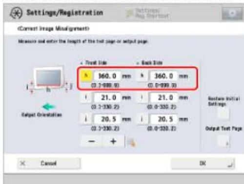
[i]: Enter the measured length of 'i' mark on the test page.
