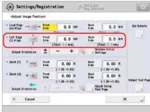
For example, if the measured length of 'l' is 21.5 mm, enter - 1.5 mm for <Left Edge (l) Align.>. For example, if the measured length of 'l' is 18.5 mm, enter + 1.5 mm for <Left Edge (l) Align.>. The difference of 1.5 mm between the measured length and the default value is corrected.
