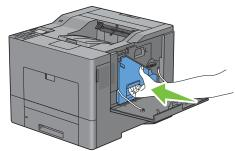
10 Turn the waste toner box lock lever 90-degrees clockwise to lock the waste toner box.
