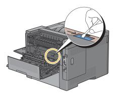
10 Make sure that the arrow marks on the transfer belt unit and the printer face each other, and then insert the unit into the printer until it clicks.
