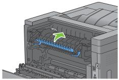
10 Press down the levers on both sides of the fusing unit, and then close the rear cover.
