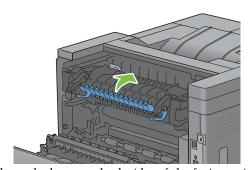
**6** Press down the levers on both sides of the fusing unit, and then close the rear cover.
