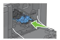
**5** Remove the cleaning rod from inside the printer.
