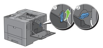
3 Grasp the handle on the waste toner box and pull it out making sure to hold it upright so that the waste toner does not spill out.
