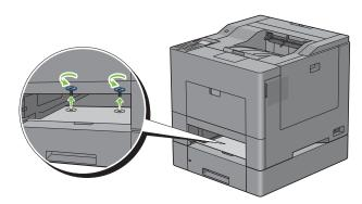
**5** Gently lift the printer off the optional 550-sheet feeder, and place it on a level surface.
