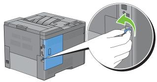
**3** Slide the left side cover towards the back of the printer.
