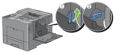
3 Grasp the handle on the waste toner box and pull it out making sure to hold it upright so that the waste toner does not spill out.
