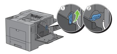
**5** Grasp the handle on the waste toner box and pull it out making sure to hold it upright so that the waste toner does not spill out.
