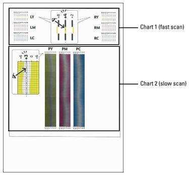
The Chart 1 is used to adjust the color registration for the fast scan direction, which is vertical to paper feed direction. The Chart 2 is used to adjust the color registration for the slow scan direction, which is horizontal to paper feed direction.
