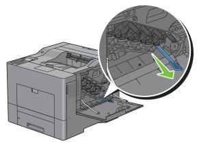
6 Insert the cleaning rod fully into one of the four holes until it clicks into the interior of the printer as illustrated below, and then pull it out.
