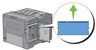
**7** Push the memory module firmly into the slot.
