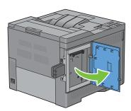
Remove the wireless adapter from the printer by releasing the adapter's hook while pushing the wireless adapter towards the front of the printer.
