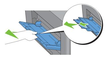
**3** Slide the width guides to the edge of the tray. The width guides should be fully extended.
