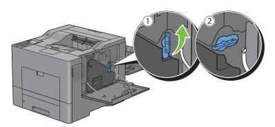
4 Grasp the handle on the waste toner box and pull it out making sure to hold it upright so that the waste toner does not spill out.
