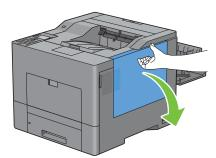
**4** Turn the waste toner box lock lever 90-degrees counterclockwise to unlock the waste toner box.
