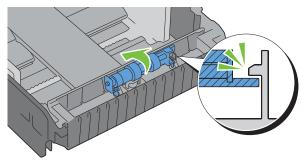
**3** Load paper in tray1, and then insert the tray into the printer and push until it stops.
