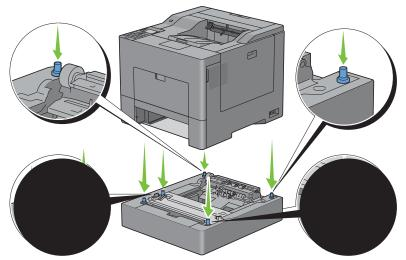
**7** Secure the optional 550-sheet feeder to the printer by tightening the two screws provided with the feeder, using a coin or similar object.
