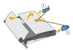
CAUTION: Ensure nothing touches or scratches the surface (black-colored film) of the transfer belt unit. Scratches, dirt, or oil from your hands on the film of the transfer belt unit may reduce print quality.
