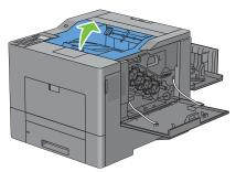
7 Put your fingers through the loops on both sides of the transfer belt unit, and then pull it out.
