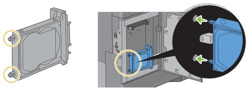
6 Attach the plastic pin and the connector to the control board, and push the hard disk firmly into place.
