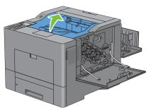
**8** Put your fingers through the loops on both sides of the transfer belt unit, and then pull it out.
