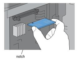
**6** Align the connector of the memory module with the slot and insert the memory module into the slot.
