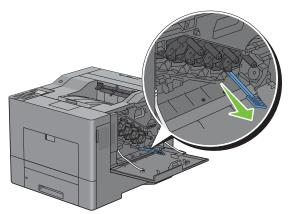
**6** Remove the cleaning pad by pressing the white tabs between your thumb and index finger.
