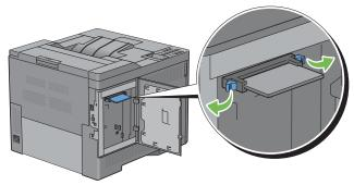
**6** Hold the memory module and pull it straight out.
