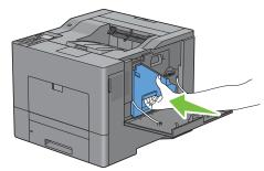
**3** Turn the waste toner box lock lever 90-degrees clockwise to lock the waste toner box.
