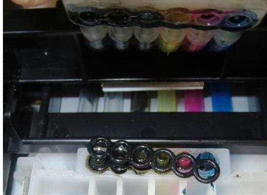
SIX-RING RUBBER CHAIN is not attached properly.
