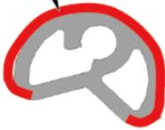
Apply grease to approx. 16 mm-wide area with the PLATE PR SUPPORT edge at the center.
