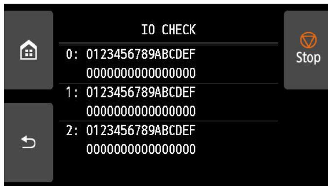
2. Switch the sensor or the switch to be diagnosed manually, and check its switching information by the display on the operation panel (0 or 1) or the beeping sounds when they are switched ON and OFF.
