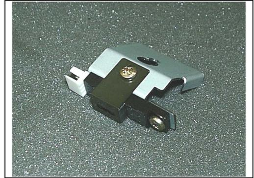
6) Remove the screw (9) top remove the Slit Plate (10).
