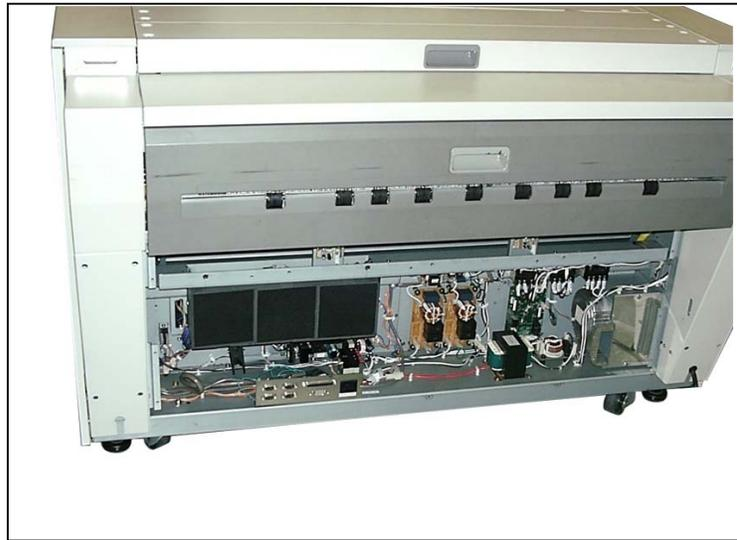
2) Remove 2 pieces of each screw (4) and Flat Washer (5) to remove the Cover 1 (6).
