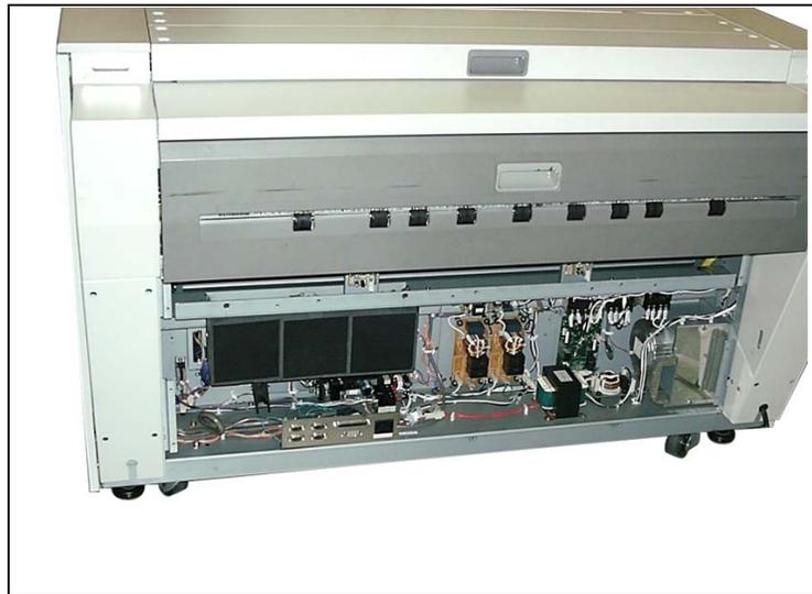
2) Remove 2 pieces of screw (4) to remove the Cover 2 (5).
