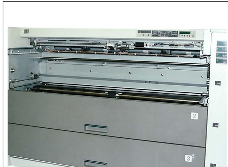
6) Remove 2 pieces of tooth washer screw (13) to remove the Cover 308 (14).
