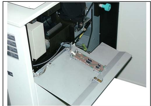
5) Disconnect the connector (8), and then remove 4 pieces of Hexagon Screw (9) to remove the **Transmission PCB** (10).
