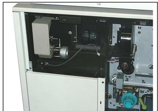
7) Remove 4 pieces of tooth washer screw (12) to remove the Bracket 562 (13).
