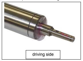
(2) Seal 1 (75) on each side should be seated in position along the bosses.
