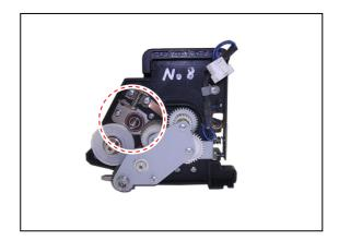
43. Make sure that the 6 screws (48) (55) (34) (52) are installed loose. If not, loosen them.
