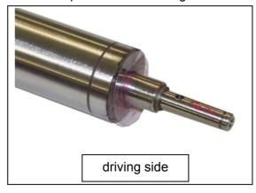
(3) Seal 1 (60) on each side should be seated in position along the boss (61).
