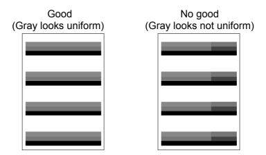
If it is still not uniform although you have fixed the Aluminium Blocks correctly, it is necessary to make focus adjustment with Spacers.
