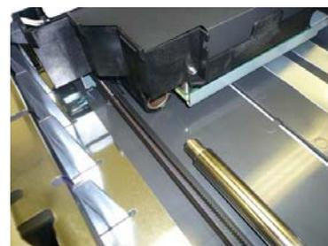
For easy removal, pull out the Carrier shaft after reinstalling the removed screw M.
