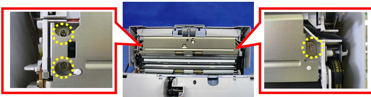
Note: Be careful not to drop the upper Sheet guide when replacing it. Otherwise, the scanning glass may be damaged.
