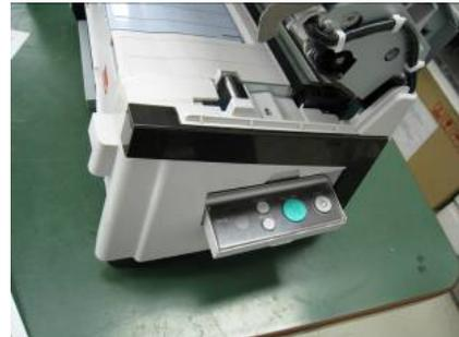
Note 4: When installing the Panel unit B, rotate the clear plastic part to fix.
