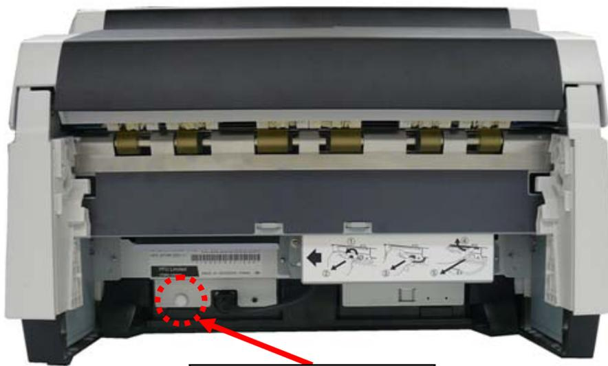
**Thumb screw inserting position**
