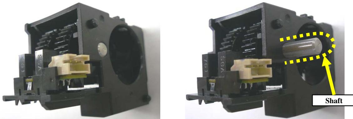
(7) Remove two screws A from the bracket to remove the BW motor.
