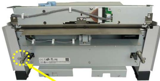
Remove a fixing screw A.
