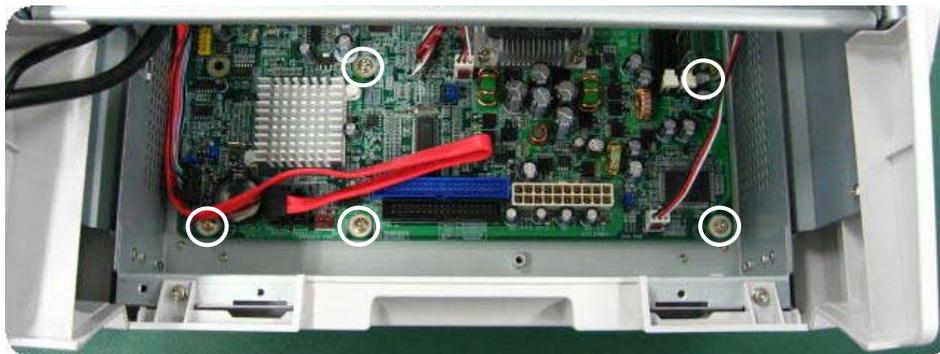
13) Disconnect three connectors of the cables at the front side of the scanner.
