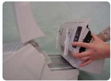
After removing two Guide Blocks, pull out the scanner section to the back.
