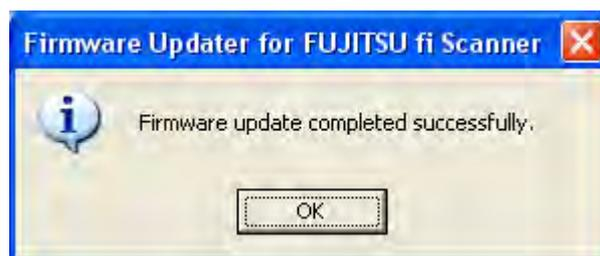
(6) After updating, confirm that the scanner firmware version is as shown in the table below. Firmware version can be confirmed in the Maintenance Mode# 6. (Refer to Section 7.1.7.)
