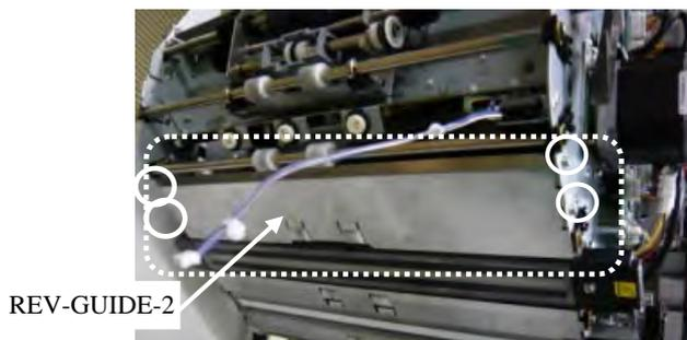
(8) Remove two screws (circles below) on the Background unit Upper, and then remove the Background unit Upper.
