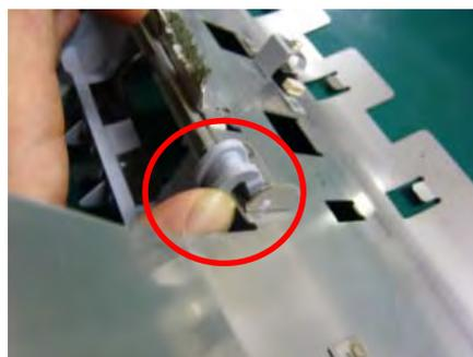
(24) Install the removed roller cover into the UPPER-GUIDE1B enclosed with the kit.
