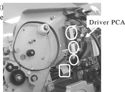
(13) Disconnect a JAM1 Sensor connector (solid square in the photo lower left).
