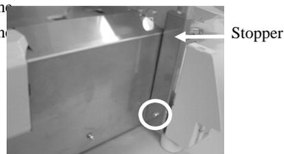
(4) Remove six (6) screws (circles in the photo below) of the SET-GUIDE (front partition) and remove the SET-GUIDE.
